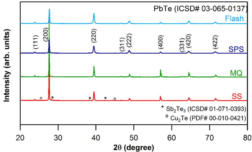
**Figure 2.** XRD patterns for different  $\text{CuPb}_{18}\text{SbTe}_{20}$  samples. For convenience, the Hybrid Flash-SPS sample is simply referred as ‘flash’ in all the figure captions in this paper.
