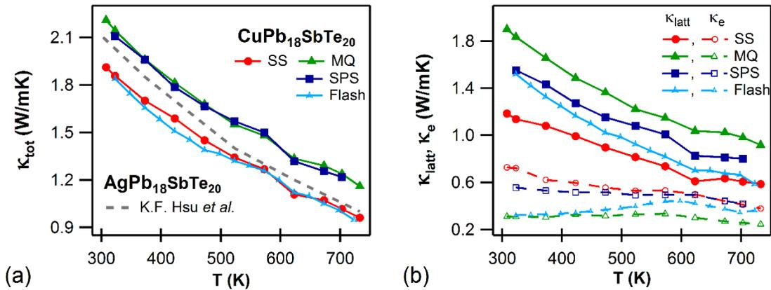
**Figure 3.** Thermal transport properties - (a) comparison of the total thermal conductivities,  $\kappa_{\text{tot}}$  of different  $\text{CuPb}_{18}\text{SbTe}_{20}$  samples vs  $\text{AgPb}_{18}\text{SbTe}_{20}$  (b) lattice,  $\kappa_{\text{latt}}$  and electronic,  $\kappa_e$  contributions to thermal transport
