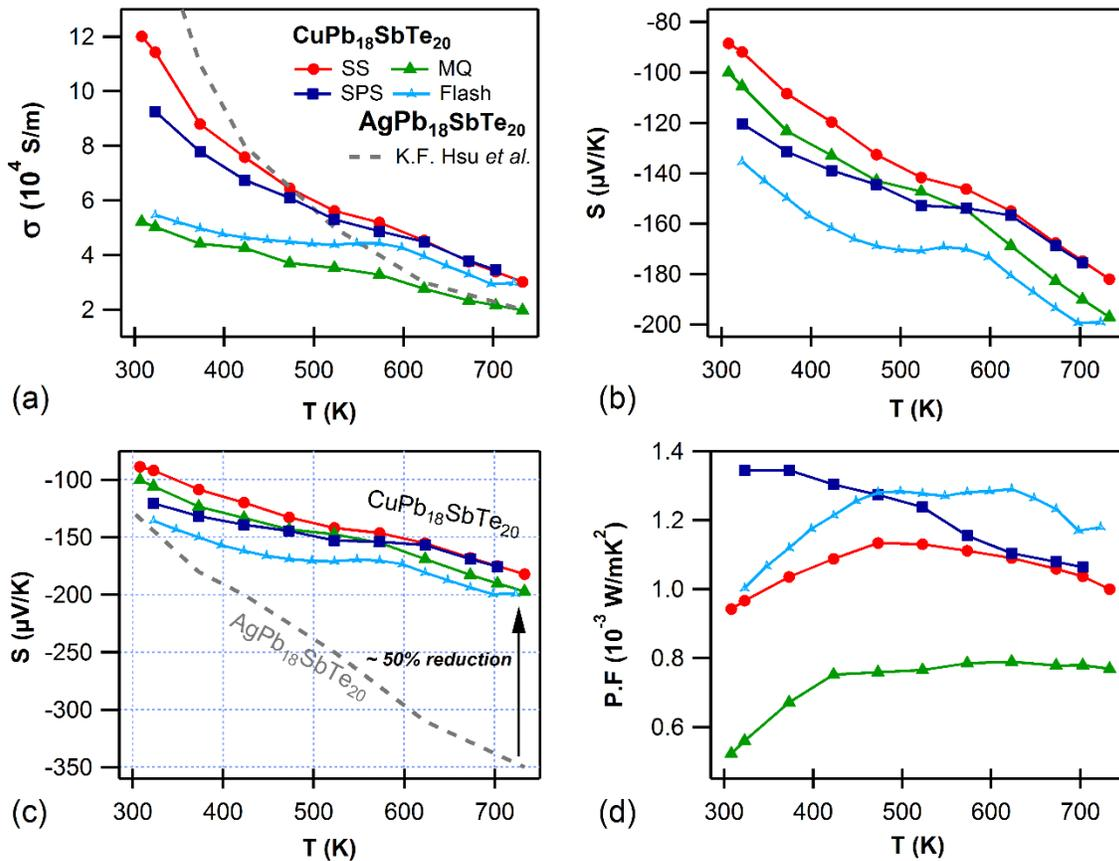
**Figure 6.** Temperature-dependent electrical transport properties for  $\text{CuPb}_{18}\text{SbTe}_{20}$  prepared by different synthesis routes - (a) electrical conductivity ( $\sigma$ ), (b) Seebeck coefficient ( $S$ ), (c) comparison of thermopower with  $\text{AgPb}_{18}\text{SbTe}_{20}$ , and (d) Power factor ( $PF = S^2\sigma$ ). Color code legend in (a) applies to all the plots here.
