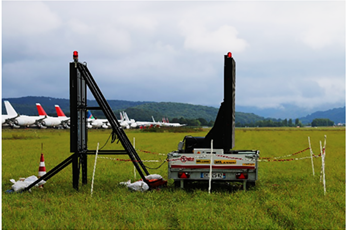
Fig 2. LED screens. The two screens placed back to back on the airport. The basis of both screens was positioned 1m above ground.
