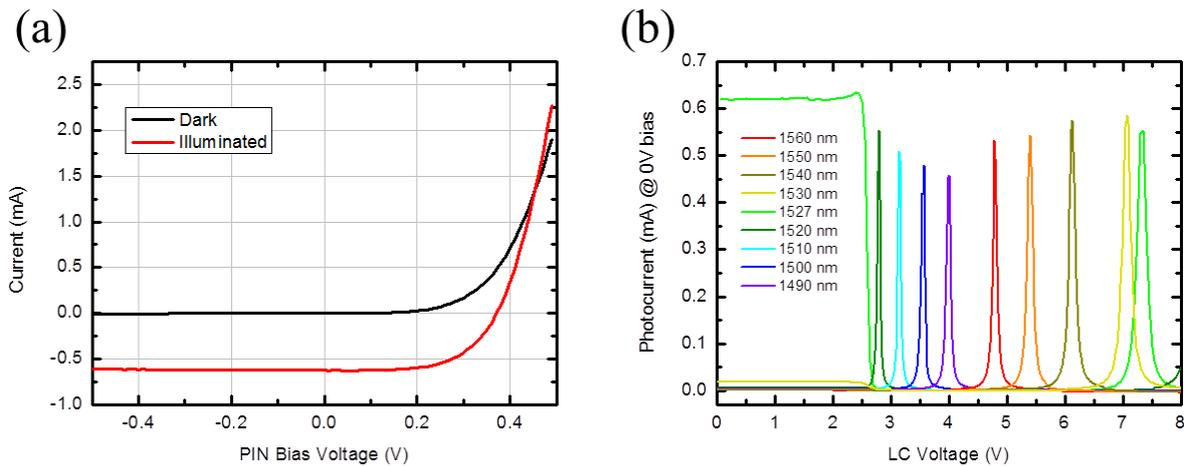
Figure 3 (a) I-V curves in the dark and under 1.4 mW illumination at 1527 nm for a  $380 \times 380 \mu\text{m}^2$  PD without any LC voltage (b) Photocurrent for the same PD related to resonant extraordinary modes vs AC voltage (2 kHz) applied on the LC microcell for different lasing wavelengths fixed at an input power of 1.4 mW.
