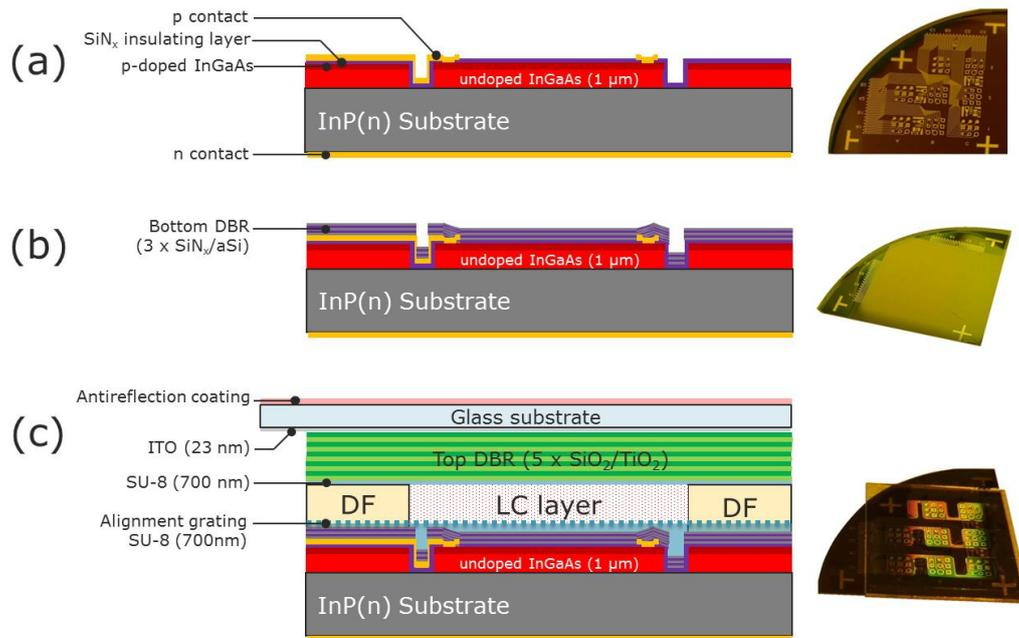
Figure 1. Cross-section views and images of the tunable PD sample at different steps of the fabrication process, (a) after PD fabrication, (b) after deposition of the aSi/SiN<sub>x</sub> bottom DBR, (c) at the end of the process.
