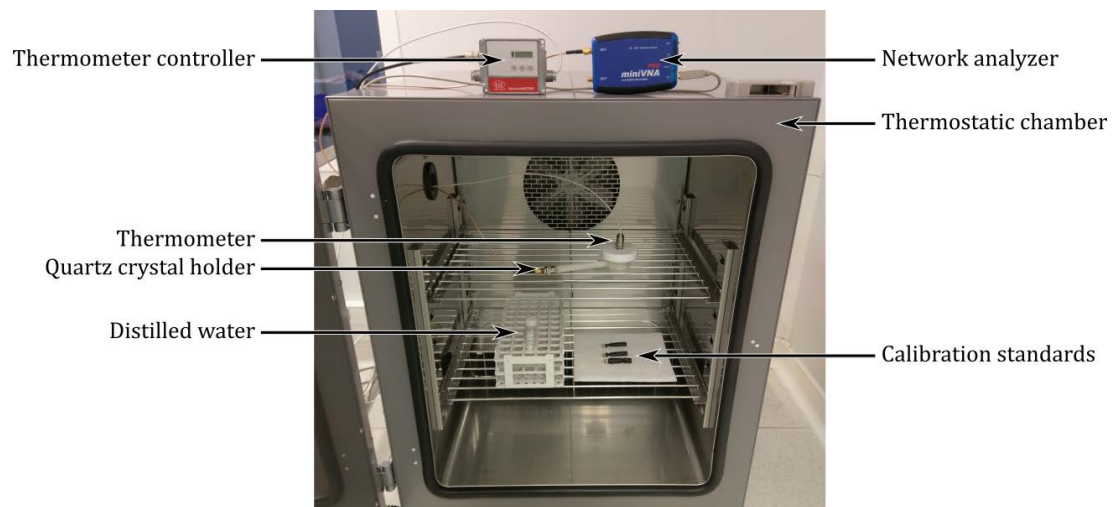
(a) Global view of the experimental setup.
