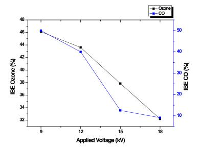
Fig.10. Variation the IBE of ozone and CO with applied voltage:  $[CHCl_3]=100 \text{ mg m}^{-3}, \ Q=6 \text{ m}^3 \text{ h}^{-1}, \ RH=50\%, \ I=20 \text{ W m}^{-2}, \ T=20 \text{ C}.$
