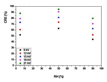
Fig.14. Influence of RH at different applied voltages on the CRE with plasma DBD/TiO $_2$ +UV: [CHCI $_3$ ]= 100 mg m $^{-3}$ , Q= 2 m $^3$  h $^{-1}$ , I= 20 W m $^{-2}$ , T= 20  $^{\circ}$ C.
