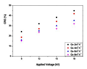
Fig.6. Influence of applied voltages at different flow rates on the CRE in plasma alone:  $[CHCI_3] = 100 \ mg \ m^{\text{-}3}, \ HR = 50 \ \%, \ T = 20 \ ^{\circ}C$
