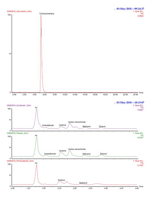
Figure 18. By-products identified by GC-MS following Trichloromethane oxidation by the different processes. Uapp= 15kV, [CHCl<sub>3</sub>]<sub>0</sub>= 50 mg m<sup>-3</sup>, Q= 2 m<sup>3</sup> h<sup>-1</sup>
