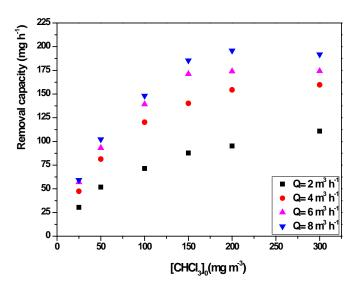
Fig 4: Influence of gas flow rates and inlet concentrations on the removal capacity of chloroform by photocatalysis alone: RH=50%,  $T=20^{\circ}C$ ,  $I=20~W~m^{-2}$ .
