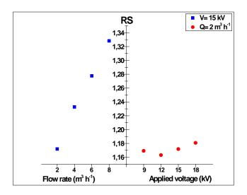
Fig.8. Variation of RS with flow rate (at V= 15 kV) and applied voltage (at Q= 2 m $^3$  h $^{-1}$ ) using three processes: [CHCl $_3$ ]= 100 mg m $^{-3}$ , RH= 50%, I= 20 W m $^2$ , T= 20  $^{\circ}$ C.
