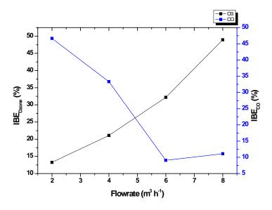
Fig.11. Variation the IBE of ozone and CO with flow rate:  $[CHCl_3]=100~mg~m^{-3},~V=18~kV,~RH=50\%,~I=20~W~m^{-2},~T=20~^{\circ}C.$
