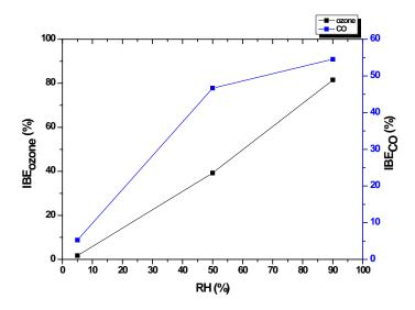
Fig.17. Variation the IBE of ozone and CO with RH:  $[CHCI_3]=100~mg~m^{\text{-}3},~Q=2~m^3~h^{\text{-}1},~V=18~kV,~I=20~W~m^{\text{-}2},~T=20~^{\circ}C.$
