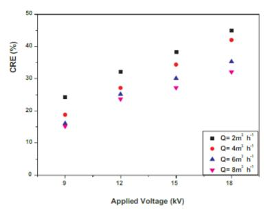
Fig. 5. Influence of applied voltages at different flow rates on the CRE in plasma alone: [CHCl3] = 100 mg m-3, HR = 50%, T = 20 °C.
