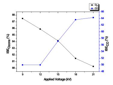
Fig.16. Variation the IBE of ozone and CO with applied voltage: [CHCl $_3$ ]= 100 mg m $^3$ , Q= 2 m $^3$  h $^1$ , RH= 90%, I= 20 W m $^2$ , T= 20  $^\circ$ C.
