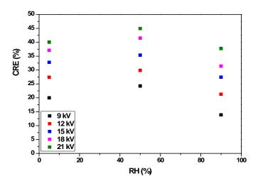
Fig.13. Influence of the RH at different voltages injected on the CRE with plasma DBD alone:  $[CHCl_3] = 100 \text{ mg m}^{-3}, \ Q= 2 \text{ m}^3 \text{ h}^{-1}, \ I= 20 \text{ W m}^{-2}.$
