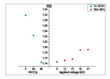
Fig.15. Variation of RS with RH (at V= 18 kV) and applied voltage (at RH= 50%) using three processes:  $[CHCl_3] = 100 \text{ mg m}^{-3}, \ Q = 2 \text{ m}^3 \text{ h}^{-1}, \ I = 20 \text{ W m}^{-2}, \ T = 20 \text{ °C}.$
