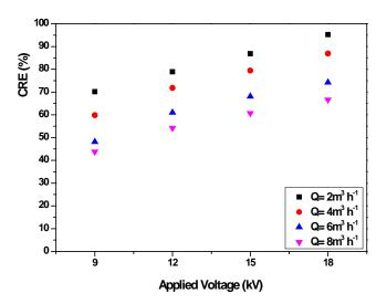
Fig.7. Influence of voltages injected at different flow rates on the CRE with plasma DBD/TiO<sub>2</sub>+UV: [CHCl<sub>3</sub>]= 100 mg m $^{\text{-3}}$ , RH= 50 %, I= 20 W m $^{\text{-2}}$ , T= 20  $^{\circ}$ C.
