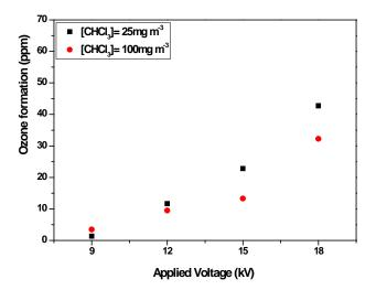
Fig.9. Influence of applied voltages at different inlet concentrations on ozone formation with plasma/TiO $_2$ +UV: HR= 50%, T= 20  $^{\circ}$ C
