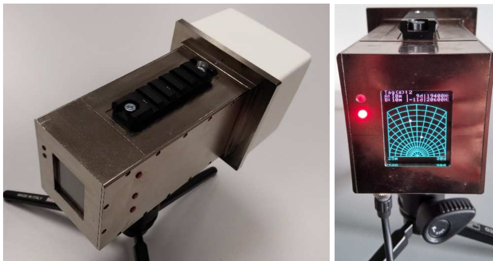
Figure 7. The designed radar equipped with an OLED display
