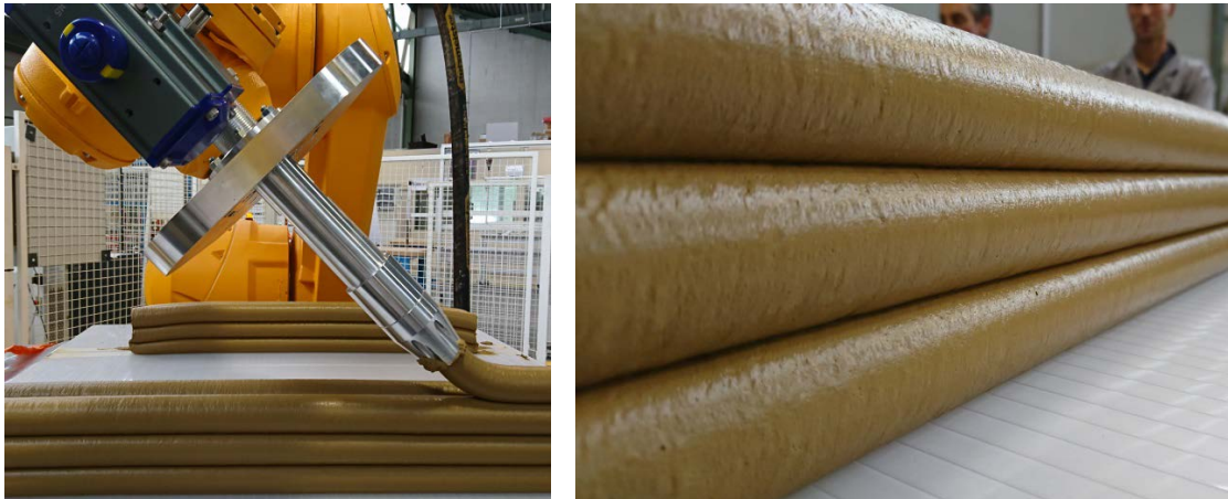
Figure 4: First performed earth printing.
