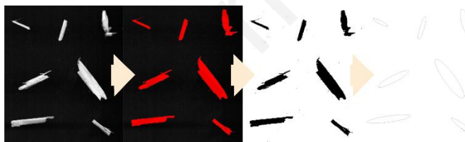
Figure 7: Image processing from left to right: scan, binarization of the image, grayscale conversion and ellipses fitting
