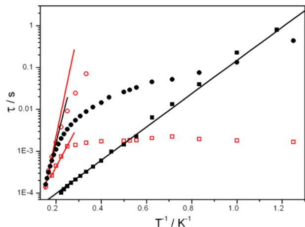
**Figure 5.** Plot of the relaxation times versus temperature for **Dy** (black symbols) and **Y:Dy** (red symbols) measured with  $H_{dc}=0 \text{ Oe}$  (squares) and  $H_{dc}=1200 \text{ Oe}$  (circles). Parameters for best fits are described in the text.
