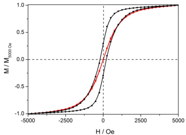
**Figure 6.** Hysteresis measurements of **Dy** and **Y:Dy** at 0.47 K with magnetic field sweep rate of 16 Oe.s<sup>-1</sup>
