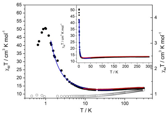
**Figure 2.** Temperature dependence of  $\chi_M T$  measured via static magnetic measurements for **Dy** (full symbol, left axis) and **Y:Dy** (empty symbol, right axis). Note the logarithmic temperature scale. *ab-initio* calculations are represented as a red line and best fit with Ising model as a blue line (see text).
