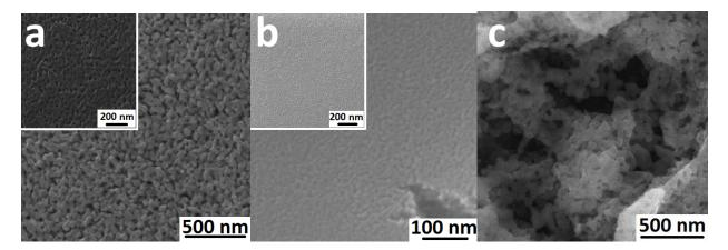
Figure 1. Surface morphology of (a) pristine  $BiVO_4$  and (inset) top-coated  $BiVO_4$  over  $TiO_2$  composite, (b) pure  $TiO_2$  and (inset) top-coated  $TiO_2$  over  $BiVO_4$  composite and (c) Nb- $BiVO_4$ .
