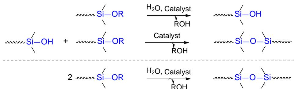
**Scheme 1.** Curing (hydrolysis and polycondensation) process of SMPs.
