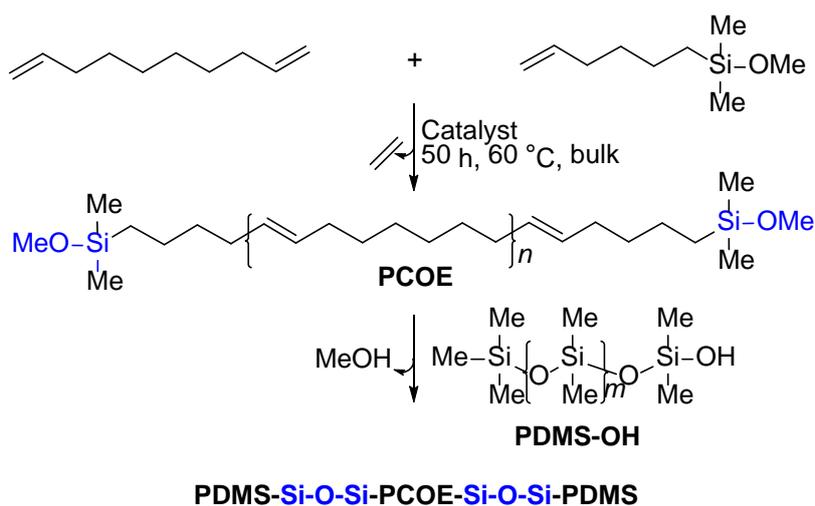
**Scheme 12.** ADMET synthesis of di(methoxysilyl) telechelic PCOE, and subsequent copolymerization with PDMS-OH.<sup>39</sup>
