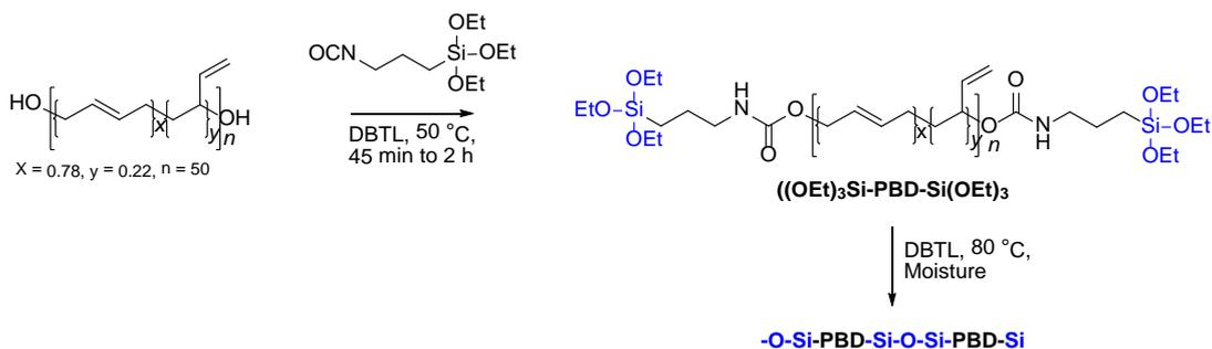
**Scheme 7.** Synthesis of bis(triethoxysilyl) telechelic PBD from dihydroxy telechelic PBD, and subsequent cross-linking.<sup>58,59</sup>
