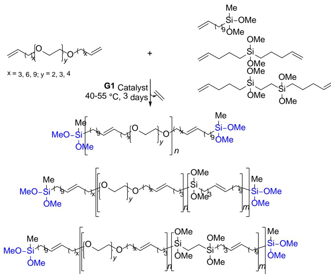
**Scheme 13.** ADMET synthesis of bis(dimethoxysilyl) telechelic polyether/carbosiloxane copolymers.<sup>44,45</sup>
