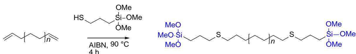
**Scheme 5.** Synthesis of bis(trimethoxysilyl) telechelic PE by thiol-ene chemistry.<sup>50</sup>
