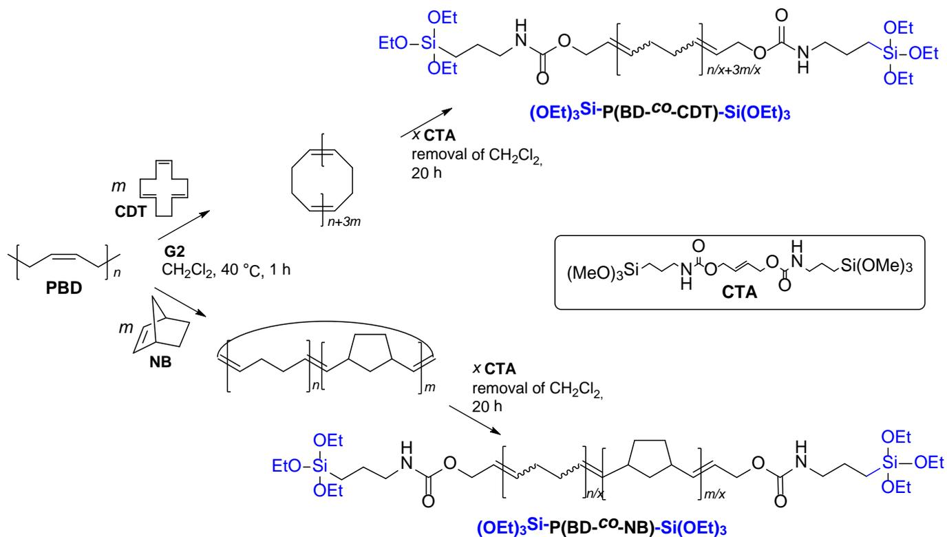
**Scheme 17.** Functional PBD CM degradation via ROMP of CDT or NB using **G2** catalyst in the presence of a bis(triethoxysilyl)diurethane-based CTA towards the formation of bis(triethoxysilyl) telechelic copolyenes.<sup>73</sup> Note that the degree of polymerization of each PCOE is only indicative, given the possible formation of side macromolecular species.
