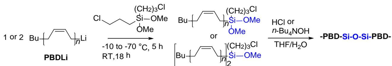
**Scheme 4.** Synthesis of  $\alpha$ -methoxysilyl end-capped PBD from PBDLi, and subsequent hydrolysis.<sup>47</sup>
