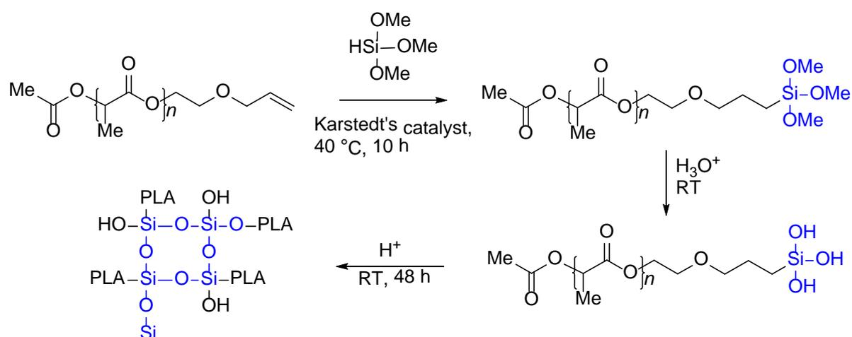
**Scheme 9.** Synthesis of  $\alpha$ -trimethoxysilyl PLA, and subsequent hydrolysis.<sup>53</sup>
