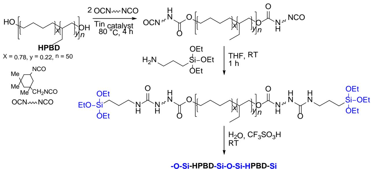
**Scheme 8.** Synthesis of bis(triethoxysilyl) telechelic HPBD from dihydroxy telechelic HPBD, and subsequent cross-linking.<sup>60,61</sup>
