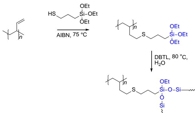
**Scheme 6.** Synthesis of triethoxysilyl functionalized PBD and subsequent cross-linking.<sup>56,57</sup>
