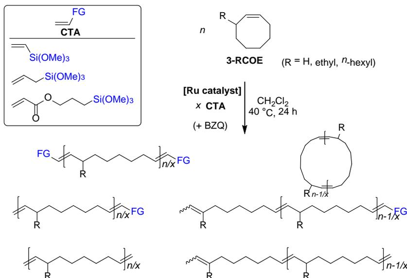
**Scheme 14.** Ruthenium catalyzed tandem ROMP/CM of 3-RCOEs using monofunctional trimethoxysilyl-alkene CTAs, showing the structural diversity of the PCOEs.<sup>70</sup> Note that the degree of polymerization of each PCOE is only indicative, given the possible formation of side macromolecular species.
