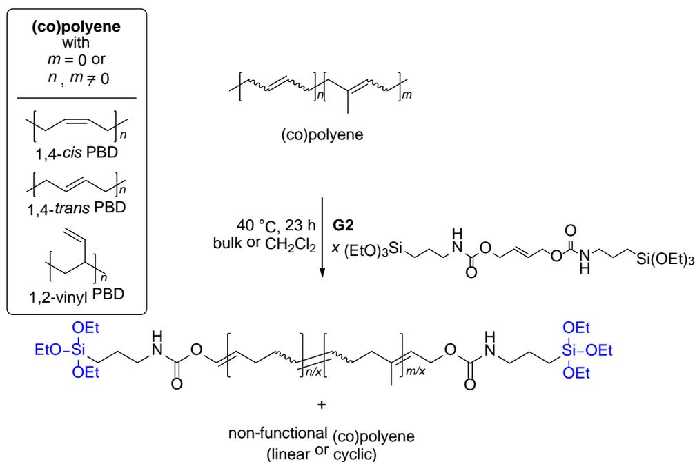
**Scheme 16.** Functional metathesis degradation reactions of PBDs ( $m = 0$ ) or P(BD-*co*-IP) ( $n$  and  $m \neq 0$ ) (co)polymers using **G2** catalyst in the presence of a bis(triethoxysilyl)diurethane-based CTA towards the formation of bis(triethoxysilyl) telechelic polyenes.<sup>73</sup> Note that the
