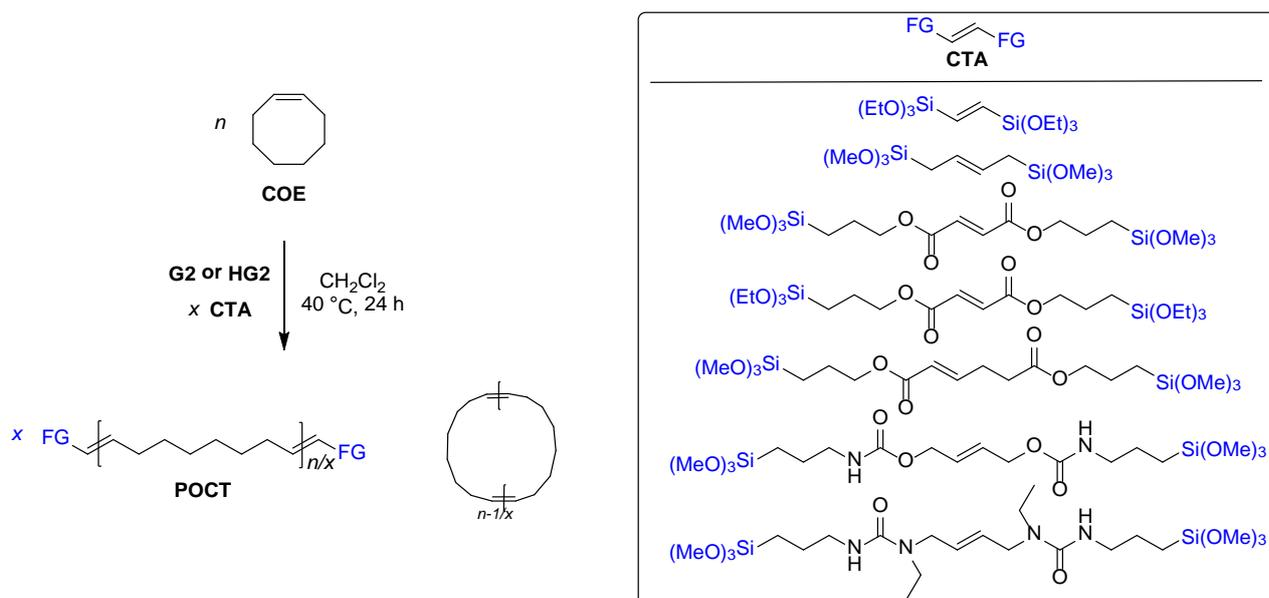
**Scheme 15.** Ruthenium catalyzed tandem ROMP/CM of COEs using difunctional trialkoxysilyl-alkene CTAs towards the formation of bis(trialkoxysilyl) telechelic PCOE.<sup>71</sup>
