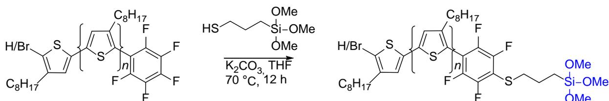
**Scheme 10.** Post-polymerization  $\alpha$ -functionalization of PTP with an  $\alpha$ -trimethoxy functional thiol.<sup>54</sup>
