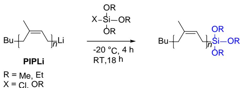
**Scheme 3.** Synthesis of  $\alpha$ -alkoxysilyl end-capped PIP from PIPLi.<sup>41</sup>
