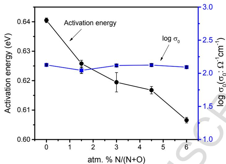
**Fig. 8.** The activation energy of the oxynitride glasses and the pre-exponential factor ( $\sigma_0$ ) of the Arrhenius equation plotted as a function of N/(N+O). The bars indicate the mathematical error from the linear regression.
