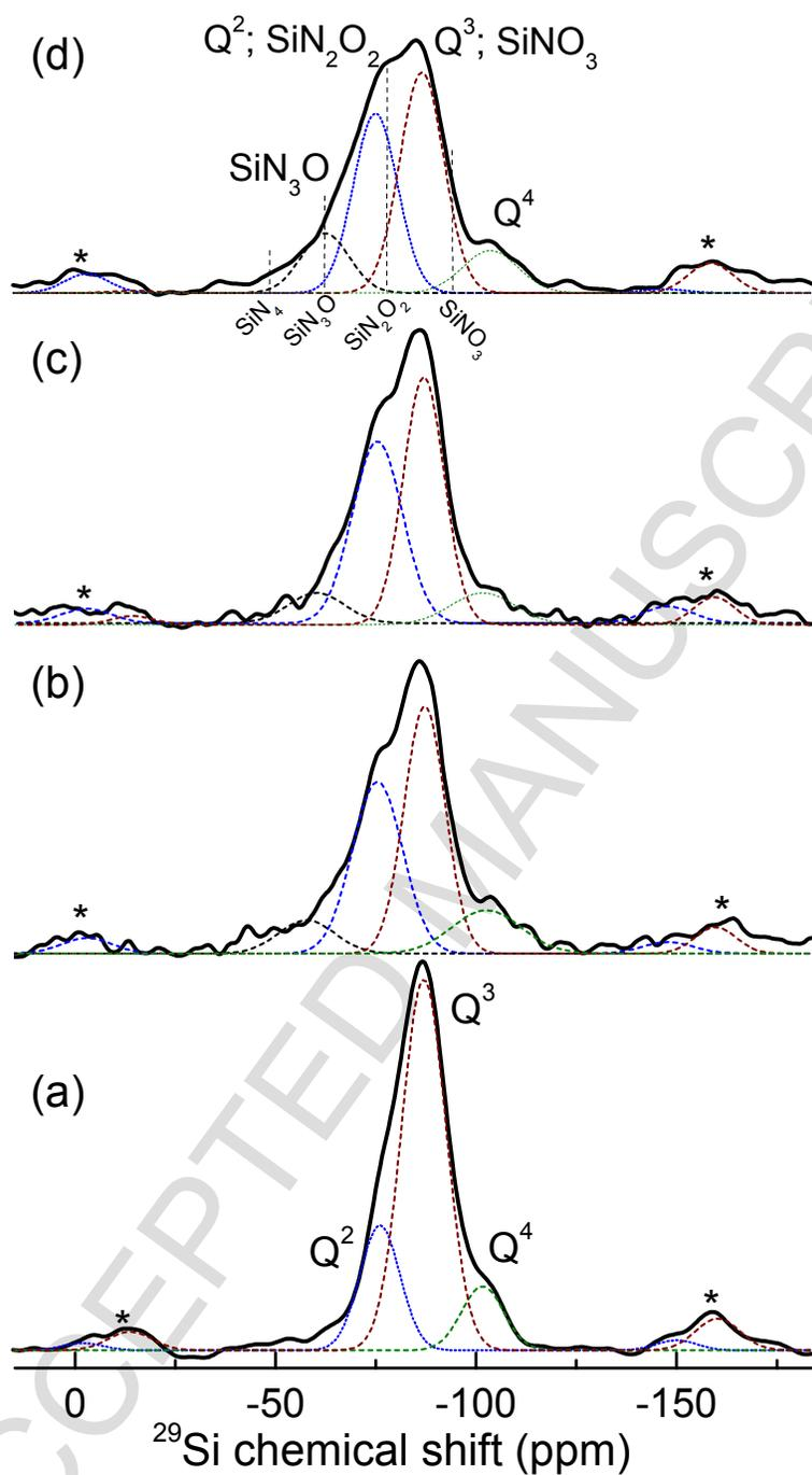
**Fig. 3.**  $^{29}\text{Si}$  NMR spectra of the glass (a) 0, (b) 3, (c) 4.5 and (d) 6 atm % N/N+O. Dotted curves: least-square fitting of Gaussian functions. Vertical lines: typical chemical shift values expected for  $\text{SiO}_{4-n}\text{N}_n$  units. Asterisks: spinning side-bands.
