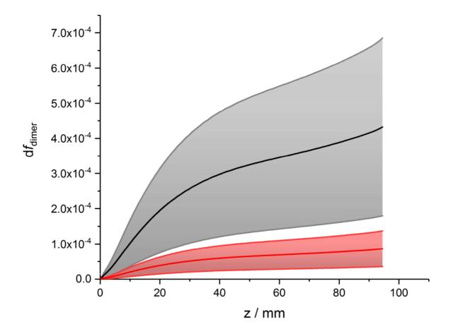
**Figure 1**. Calculated  $df_{dimer}$  as a function of the distance along the 52 K Laval nozzle axis (z) from throat to nozzle exit. The black line assumes 0.5% of the gas flow consists of methanol (the maximum used with this nozzle) whilst the red line assumes 0.1% of the total gas flow consists of methanol. Error bars are assigned through varying the binding energy of the dimer as described in Section 2 of the manuscript.
