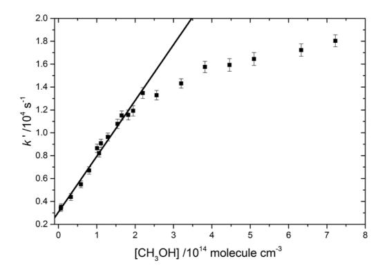
**Figure 4.** Experimental results (squares) of the pseudo-first order loss of OH (k') as a function of the methanol concentration (bimolecular plot) using the University of Leeds Laval apparatus at 56 K, together with a linear-least squares fit to the linear portion of the data (solid line), from which the bimolecular rate coefficient for the reaction of OH with methanol was determined. The results were reported in Gómez-Martín et al.<sup>3</sup>
