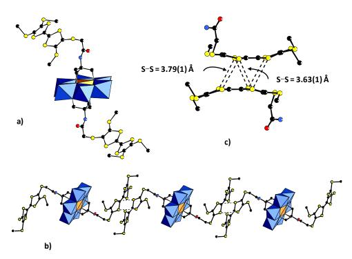
**Figure 3**. Structure of **TTF-MnMo<sub>6</sub>-TTF**; a) view of the molecular structure, b) chain formed by supramolecular interactions between the molecules, c) side view of the TTF moieties in interaction within the chain; black spheres = C, red spheres = O, yellow spheres = S, blue spheres = N, blue octahedra =  $MoO_6$ , orange octahedra =  $MnO_6$ ; hydrogen atoms have been omitted for clarity.
