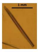
**Figure 1.** Picture of a needle-like single crystal of [Er₂(dcpa)₃(H₂O)₅⋅3H₂O]∞.
