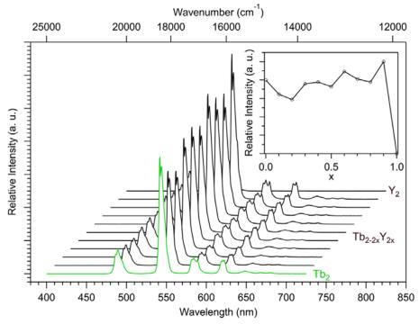
**Figure 7.** Emission spectra of  $[Tb_{2-2x}Y_{2x}(dcpa)_3(H_2O)_5 \cdot 3H_2O]_{\infty}$  with  $0 \le x \le 1$  versus x ( $\lambda_{exc} = 302$  nm) at 293 K. In inset: maximum intensities versus x.
