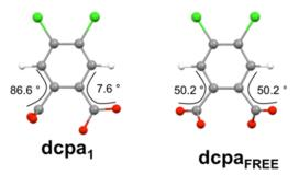
**Scheme 3.** Left: Geometrical arrangement of dcpa $_1$  extracted from the solid state structure of  $[Er_2(dcpa)_3(H_2O)_5\cdot 3H_2O]_{\infty}$ . Right: DFT fully-optimized arrangement dcpa $_{FREE}$ . Calculated dihedral angles between the phenyl ring and the carboxylate groups are indicated.
