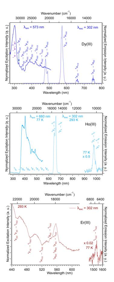
**Figure 6.** Solid state excitation and emission spectra of  $[Ln_2(dcpa)_3(H_2O)_5 \cdot 3H_2O]_{\infty}$  with Ln = Tb(III), Dy(III), Ho(III) or Er(III) (from top to bottom) at 77 K or 293 K.
