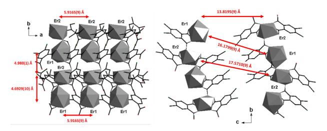
**Figure 3.** Intermetallic distances between lanthanide ions that belong to the same molecular plane (left) or to adjacent planes (right) in  $[Er_2(dcpa)_3(H_2O)_5 \cdot 3H_2O]_{\infty}$ .
