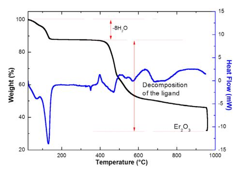
**Figure 5.** TGA/DSC of  $[Er_2(dcpa)_3(H_2O)_5 \cdot 3H_2O]_{\infty}$  between room temperature and 950 °C under nitrogen atmosphere. At 950 °C, nitrogen is replaced by air in order to insure complete decomposition.
