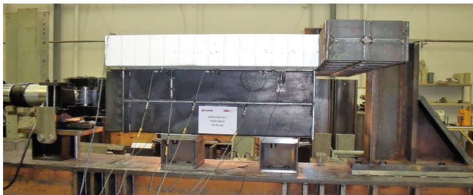
Figure 3: Side view of push-out test setup.
