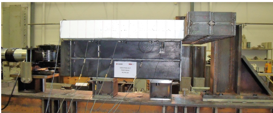
Figure 3: Side view of push-out test setup.
