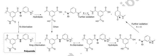
Figure 1: Proposed general mechanism of chlorine attack on polyamide: N-chlorination, direct ring-chlorination, Orton rearrangement, and hydrolysis [4].
