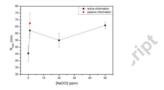
Figure 9: The root-mean-square roughness ( $R_{RMS}$ ) of the actively and passively chlorinated membranes as function of NaOCl concentration in the feed. Values shown are the average of at least 3 replicates, each of which was obtained by scanning a 5x5  $\mu$ m<sup>2</sup> surface area.
