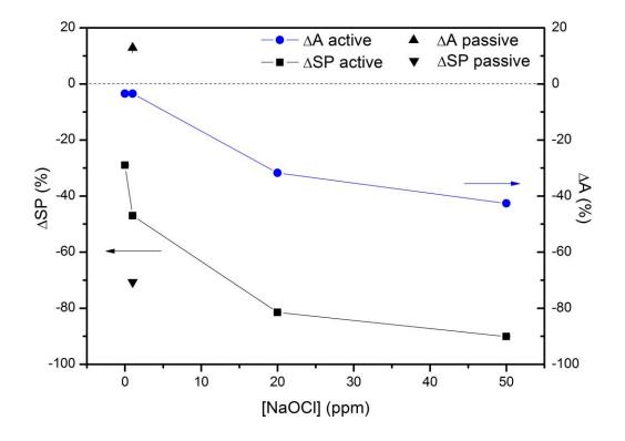
Figure 11: Change in membrane permeability coefficient (A) and salt passage (SP), based on total ions, of BW30 8" membrane elements before and after the chlorination step. Filtration conditions of standard tests: NaCl (2000 ppm), iso-propanol (100 ppm) and boric acid (5 ppm) in RO permeate at 15.5 bar, 25 °C, pH8 and a recovery of 15%. Values are based on average values of SP and A of pre- and post-Cl-STs.
