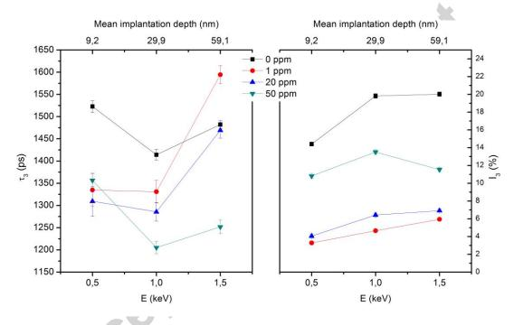
Figure 12: o-Ps lifetime  $(\tau_3)$  and intensity  $(I_3)$  as function of different positron implantation energies and corresponding implantation depths. Data from one measurement point of all actively chlorinated membranes with 0, 1, 20 and 50 ppm NaOCl in the feed.
