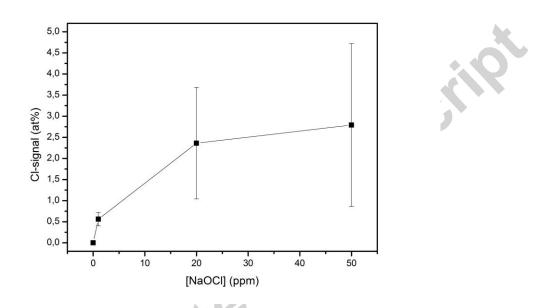
Figure 6: XPS organochlorine (C-Cl) signal as a function of the NaOCl concentration in the feed, based on 4 measurements. Chlorine in the reference (0 ppm) membrane was only present as chloride (Cl<sup>-</sup>), while all other actively chlorinated membranes contained both Cl<sup>-</sup> and covalently bound organochlorine. No Cl in any form could be detected for the passively chlorinated membrane.
