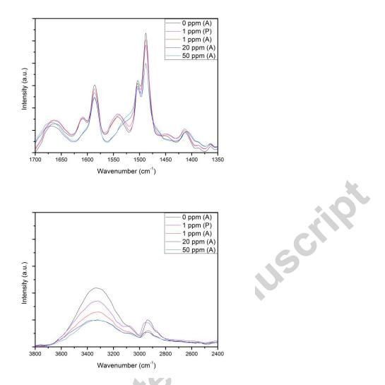
Figure 4: Representative ATR-FTIR spectra for the reference membrane (0 ppm) and chlorinated membranes at pH4, during 2 h, at 1, 20 and 50 ppm NaOCl. (top) Emphasis on characteristic PA peaks. (bottom) Emphasis on characteristic removable coating layer peaks. (A) and (P) denote active and passive chlorination, respectively.
