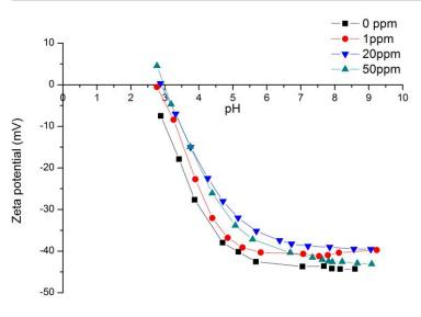
Figure 10: Zeta-potential of the actively chlorinated membranes as function of NaOCl concentration in the feed.
