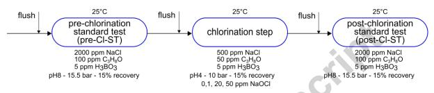
Figure 3: Schematic diagram of the active chlorination protocol of DOW FILMTEC<sup>TM</sup> BW30 elements at pilot-scale. All three steps (pre-chlorination standard test, chlorination step, post-chlorination standard test) were executed in recirculation mode.
