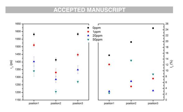
Figure 13: o-Ps lifetime ( $\tau_3$ ) and intensity (I<sub>3</sub>) at 1 keV (~ mean implantation depth of 30 nm) as function of different sample positions for all actively chlorinated membranes with 0, 1, 20 and 50 ppm NaOCl in the feed. Values are from one measurement point and 3 different positions of each sample were probed.
