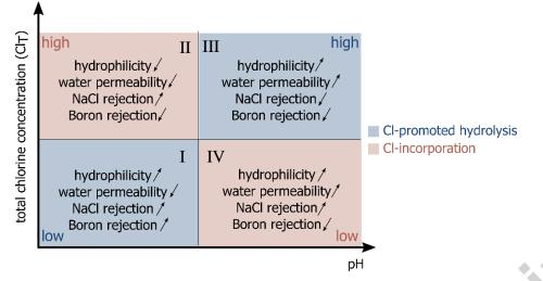
**Figure 2:** Main effects of pH and chlorine concentration on membrane performance and characteristics, adapted from [14].
