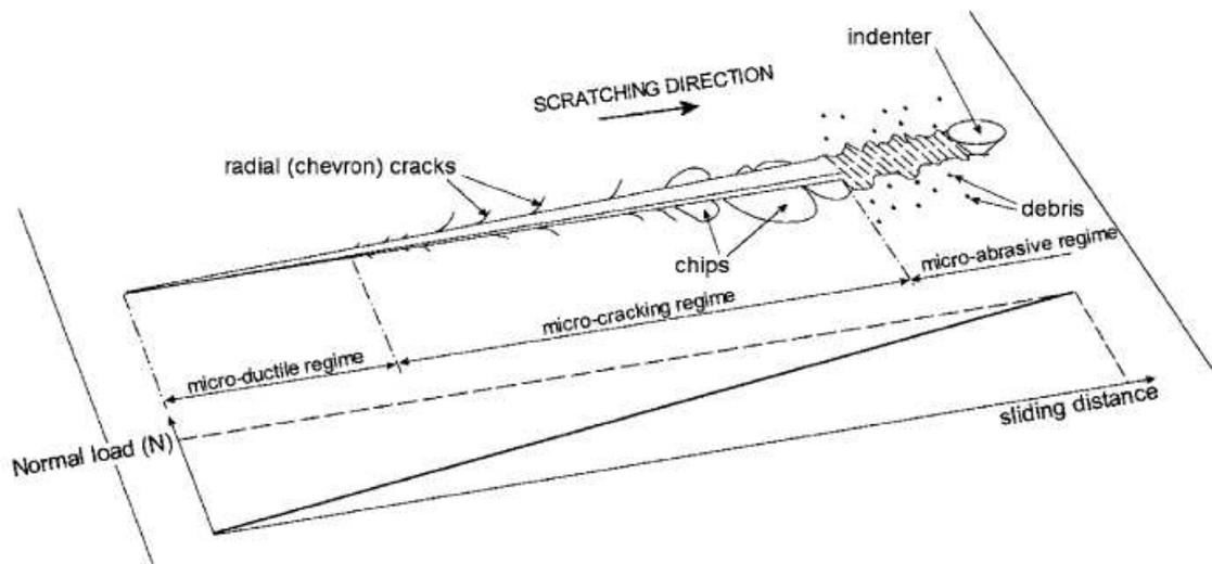
**Fig. 1:** Typical scratch obtained on a soda-lime-silica glass. [3]
