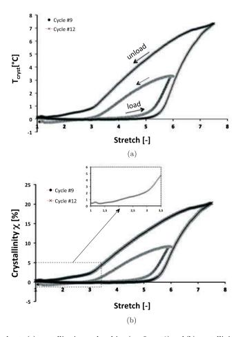
**FIGURE 4** Temperature change due to (a) crystallization and melting (see Step #3) and (b) crystallinity (see Step #4) in relation to the stretch
