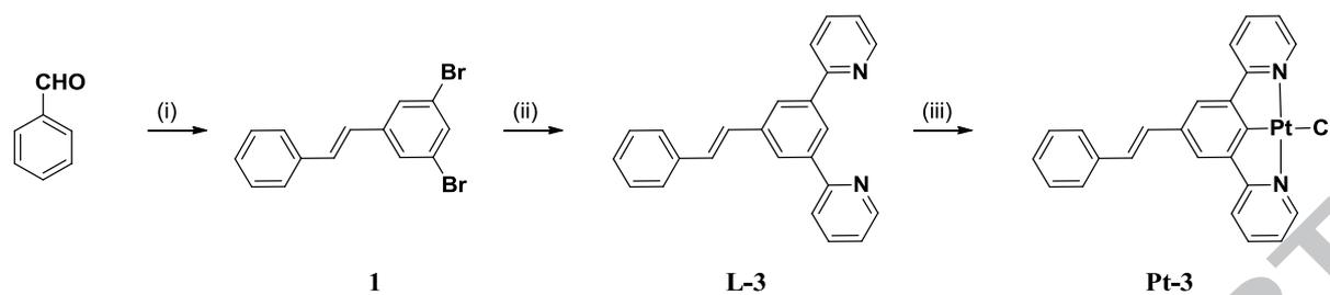
**Scheme 1.** Reagents and conditions: (i) Diethyl 3,5-dibromobenzylphosphonate, *t*-BuOK, THF, Ar, 0°C, then rt, 15 h, 58% yield; (ii) 2-(tri-*n*-butylstannyl)pyridine, LiCl, PdCl<sub>2</sub>(PPh<sub>3</sub>)<sub>2</sub>, toluene, 110°C, 48 h, 48% yield; (iii) K<sub>2</sub>PtCl<sub>4</sub>, AcOH, 118°C, 48 h, 77% yield.
