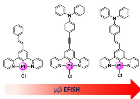
The novel easily-prepared platinum(II) complex with a cyclometallated 5-styryl-1,3-di(2-pyridyl)benzene is characterized by a good second-order NLO response, as determined in solution by the EFISH technique and it is a good candidate for application in photonics.
