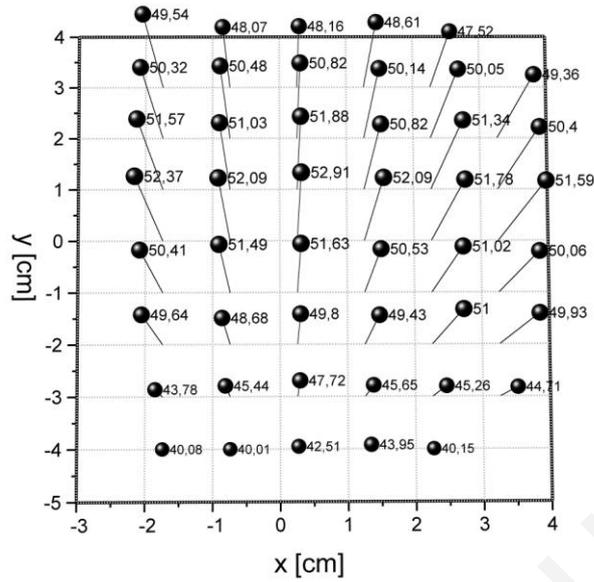
Fig. 3 The composition of  $\text{As}_2\text{S}_3$  film obtained from EDS. The numbers indicate amount of As (at. %) in the film.
