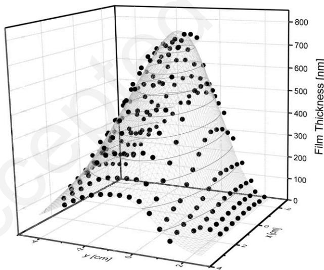
Fig. 2 Thickness distribution and fit of  $As_2S_3$  film
