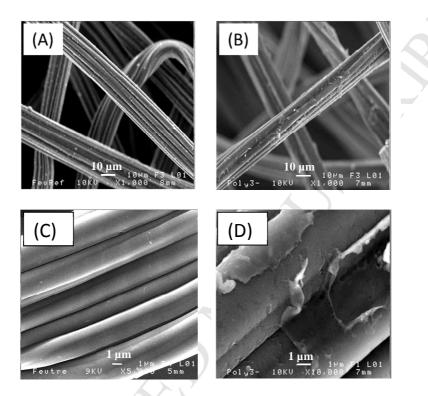
**Fig. 9.** SEM images of (A,C) blank carbon felt; (B, D) Ru-polymer deposited onto the fibers constituting the carbon felt.
