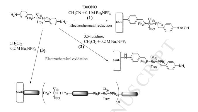
**Fig. 1**: Three strategies for surface functionalization at a glassy carbon electrode (GCE). (1) electrochemical reduction of diazonium salt produced from 1 mM Ru-complex in  $CH_3CN + 6$  mM of t-BuONO, (2) electrochemical oxidation of 1 mM Ru-complex in  $CH_2Cl_2 + 50$  mM of 3,5-lutidine and (3) electropolymerisation of 1 mM Ru-complex in  $CH_2Cl_2$
