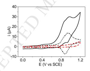
**Fig. 5**. Cyclic voltammetries of  $[Ru(trans-PN)_2(trpy)Cl]^+Cl^-$  in  $CH_2Cl_2 + 0.2$  M NBu<sub>4</sub>PF<sub>6</sub> in the absence (dotted line) and in the presence (solid line) of 50 eqs. 3,5-lutidine. Signal of 3,5-lutidine alone (red dashed line) is provided for sake of comparison. Scan rate is 100 mV s<sup>-1</sup>.
