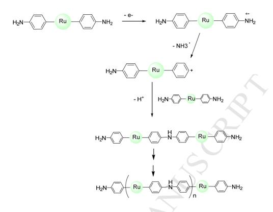
**Fig. 10.** Scheme of mechanistic pathways proposed for oxidative electro-polymerization of  $[Ru(trans-PN)_2(trpy)Cl]^+Cl^-$  complex.
