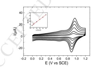
**Fig. 7**. Electrochemical behavior in  $CH_2Cl_2$  (+ 0.2 M NBu<sub>4</sub>PF<sub>6</sub>) of an electrode modified through oxidation of [Ru(*trans* $-PN)_2(trpy)Cl]^+Cl^-$  in the presence of 50 eqs. 3,5-lutidine at different scan rates (0.05 to 0.5 Vs<sup>-1</sup>). Insert: linear variation of the anodic peak current intensity of the modified electrode as a function of the scan rates.
