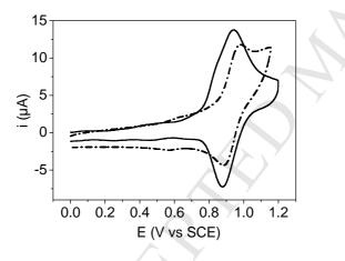
**Fig. 3.** Cyclic voltammetry of a millimolar solution of  $[Ru(trans-PN)_2(trpy)Cl]^+Cl^-(-)$  and  $[Ru(trans-PPh_3)_2(trpy)Cl]^+Cl^-(- -)$  in  $CH_2Cl_2 + 0.2$  M NBu<sub>4</sub>PF<sub>6</sub> at a GC electrode. v= 100 mV s<sup>-1</sup>
