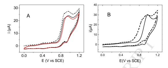
**Fig. 6.** Cyclic voltammograms of  $[Ru(trans-PN)_2(trpy)Cl]^+Cl^-$  in  $CH_2Cl_2 + 0.2$  M NBu<sub>4</sub>PF<sub>6</sub> at a glassy carbon surface in the presence of 50 eqs. of 3,5-lutidine **A**) 1<sup>st</sup> (dotted line), 2<sup>nd</sup> (black solid line), 5<sup>th</sup> (red solid line) scans and **B**) before (dashed line) and after (solid line) controlled-potential electrolysis at 0.86 V. Scan rate is 100 mV s<sup>-1</sup>.
