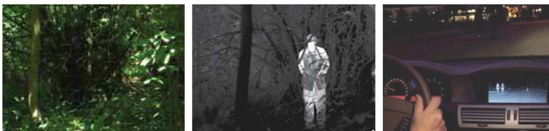
Fig. 2. Visible image (left), same image in the infrared (center), night driving assistance (right).
