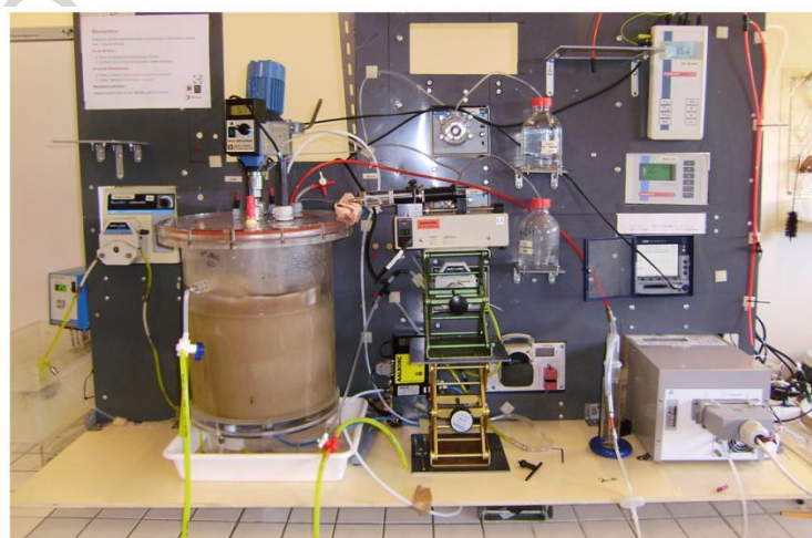
Figure 1 Semi-continuous 10 L stirred tank reactor for toluene biodegradation
