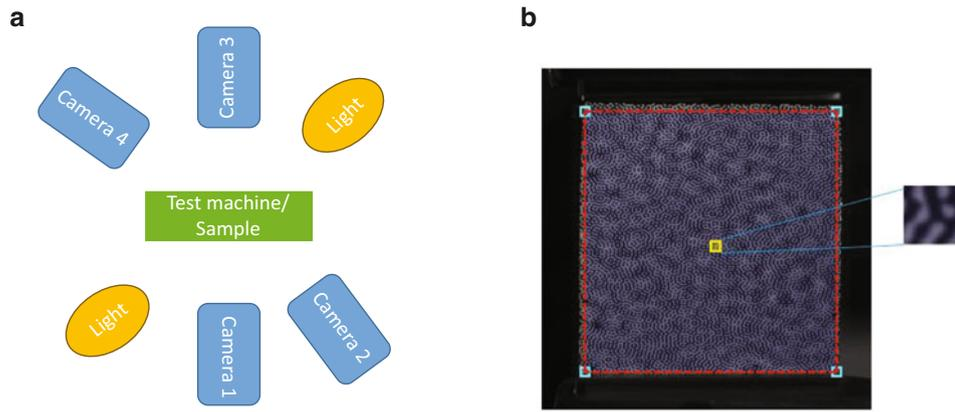
**Fig. 47.1** Schematic of the back-to-back camera test configuration showing (a) the position of the cameras and lights relative to the test machine and (b) a sample image of the elastomer with the speckle pattern applied. The *small block* shows a representative subset
