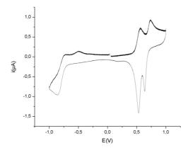
**Figure 1** Cyclic voltamogramm of  $[Au(nPr-thiazdt)_2]^{1-}$  **3-nPr** in CH<sub>2</sub>Cl<sub>2</sub> with NBu<sub>4</sub>PF<sub>6</sub> 0.1 M as electrolyte, E in V *vs* SCE, Pt electrode, scan rate 100 mV.s<sup>-1</sup>.
