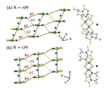
**Figure 7**. The overlap interactions a,  $b_1$  and  $b_2$  in the layers (left), and detail of the intra-stack overlap **a** (right) in (a) **4-nPr** and (b) **4-cPr**. The dotted lines are only a guide to the eyes to visualize interacting molecules.
