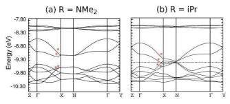
**Figure 4** Calculated band structure of the gold complexes a) **4-NMe**<sub>2</sub> and b) **4-iPr** with the HOMO-1(4 bands), SOMO (4 bands marked with red asteriks) and LUMO (4 bands) where  $\Gamma = (0, 0, 0)$ ,  $X = (\frac{1}{2}, 0, 0)$ ,  $Y = (0, \frac{1}{2}, 0)$ ,  $Z = (0, 0, \frac{1}{2})$ , and  $N = (\frac{1}{2}, 0, \frac{1}{2})$  of the Brillouin zone of the triclinic lattice. The dashed line in **4-iPr** refers to the Fermi level assuming a metallic filling of the levels.
