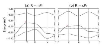
**Figure 8.** Band structures of the (a) **4-nPr** and (b) **4-cPr** gold complexes. The SOMO bands are marked with a red asterisk.  $\Gamma = (0, 0, 0), X = (\frac{1}{2}, 0, 0), Y = (0, \frac{1}{2}, 0), A = (\frac{1}{2}, -\frac{1}{2}, 0)$  of the Brillouin zone of the monoclinic lattice. The dashed line refers to the Fermi level assuming a metallic filling of the levels.
