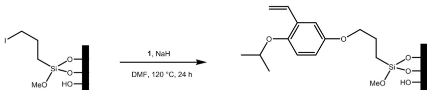
Fig. 6. Grafting of 1 onto the silylated grafted membrane.
