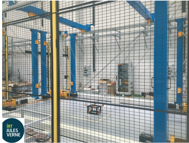
Fig. 1: CAROCA prototype: a reconfigurable CDPR (Courtesy of IRT Jules Verne, Nantes)
