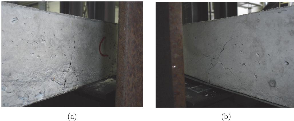
Figure 14: Cracking of concrete at both sides of the composite beam specimen
