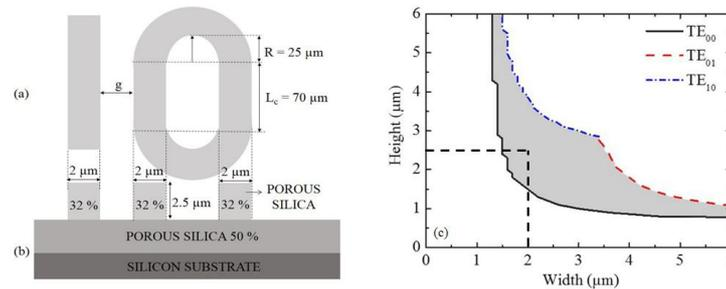
Figure 1: Schema of a top view (a) and a cross section (b) of the porous silica racetrack MR. (c) Solutions of the Maxwell equations for the  $TE_{00}$ ,  $TE_{01}$  and  $TE_{10}$  modes as a function of the porous silica ridge waveguide dimensions.
