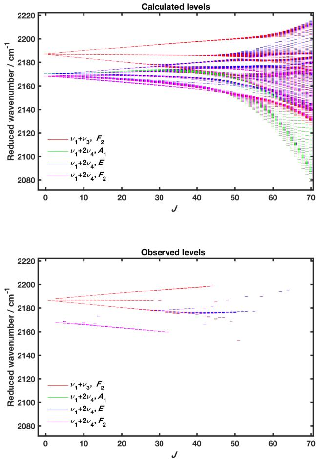
Figure 12: Observed and calculated reduced rovibrational energy levels for the  $\nu_1 + (\nu_3/2\nu_4)$  region, compared to the simulation. “Observed” levels correspond to those reached by assigned transitions. The colors represent the mixings between the different sublevels.
