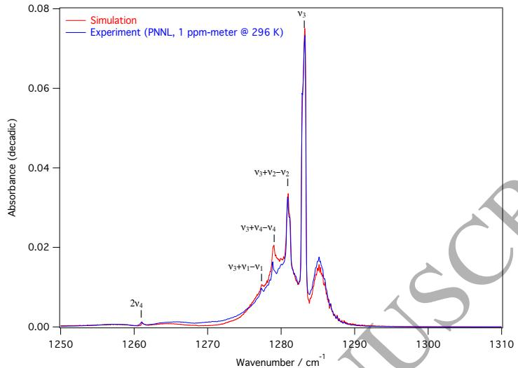
Figure 14: PNNL (see text and Ref. [46]) spectrum of the  $\nu_3$  region, including hot bands, at low resolution, compared to the simulation.
