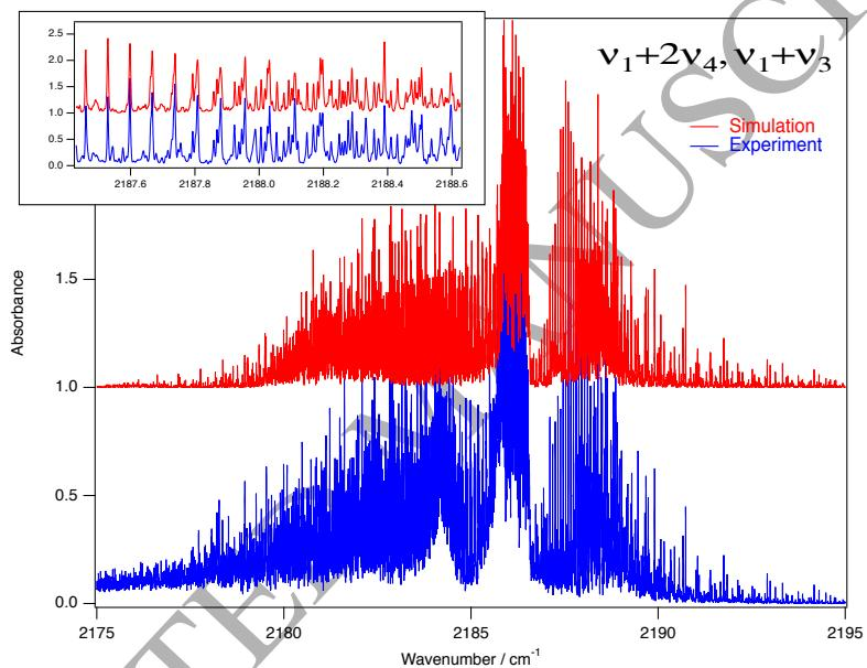
Figure 11: Measured spectrum of the  $\nu_1 + (\nu_3/2\nu_4)$  region at 295 K and 0.5 Torr, compared to the simulation. The insert details a part of the  $R$  branch. The strong  $Q$  branch near 2183  $\text{cm}^{-1}$  is the  $\nu_1 + \nu_3 + \nu_2 - \nu_2$  hot band, which is not simulated here.
