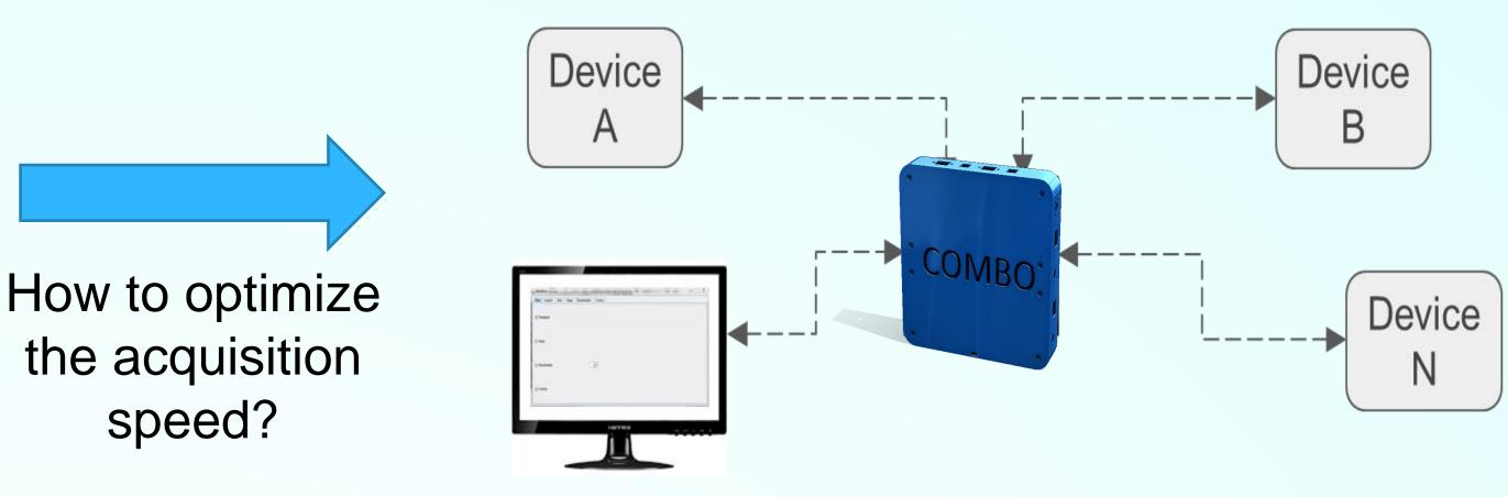
(i) microcontroller entirely dedicated to multidimensional acquisition process; (ii) direct communications which do not require any device software driver to operate and provides various types of interfaces (COM, TTL, and USB) with the possibility to add many others;
