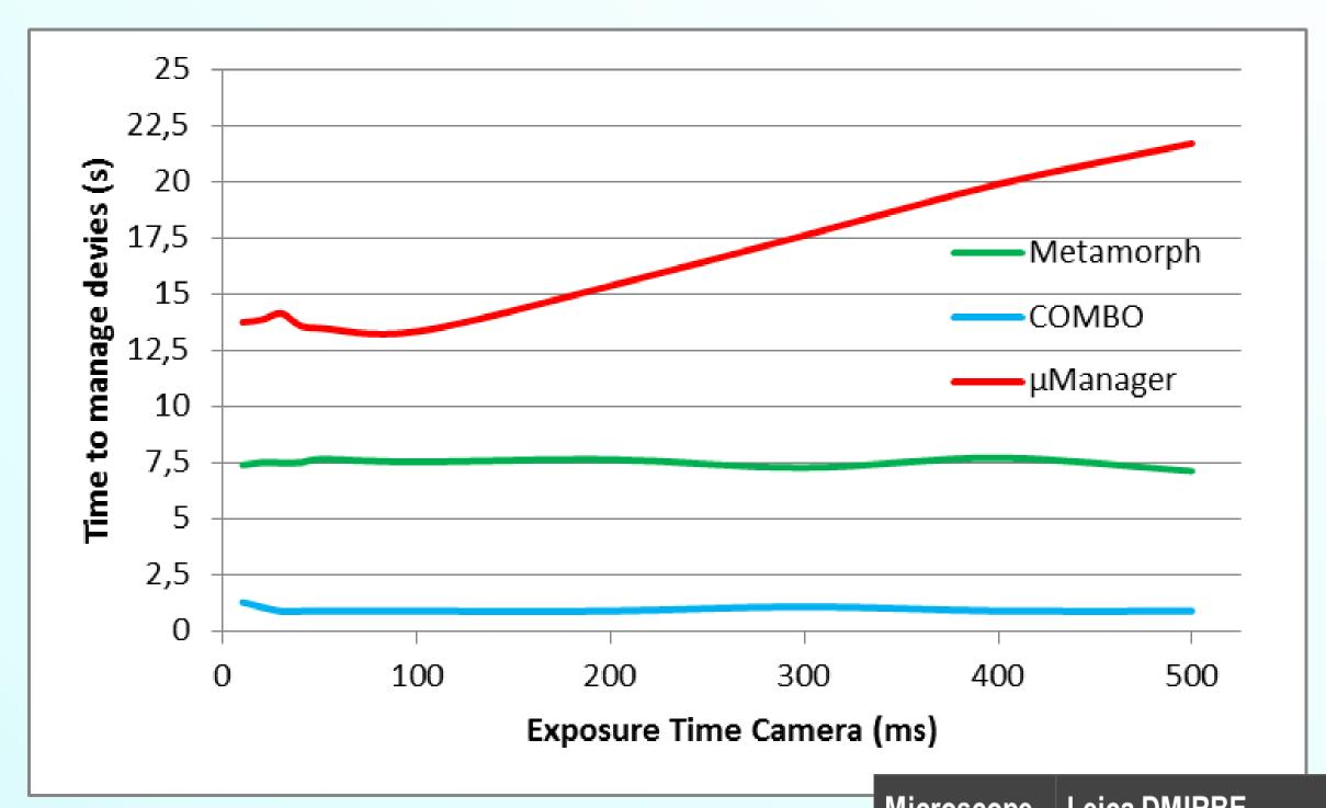
figure represents the time to manage devices during an acquisition of 22 images for 2 illumination settings and 11 Z-stack.
