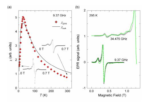
**Figure 3.** (a) The temperature dependence of the X-band (9.37 GHz) EPR susceptibility (intensity) compared to the bulk susceptibility. The corresponding high- and low-temperature spectra are displayed. (b) Comparison of the X- and Q-band EPR spectra at RT (grey symbols) and corresponding fits (green lines) of the  $Cr^{III}\cdots Cr^{III}$  dimer model (see text for details).
