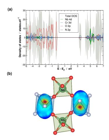
**Figure 5.** (a) Total DOS and projected PDOS onto specific atomic orbitals calculated in the HSE06 approximation. Carbon and hydrogen atoms are not represented for simplicity. (b) Representation of the local environment of the square shaped { $Cr_2(\mu-O)_4Nb_2$ } core. For each  $Cr^{III}$  ions the single-ion anisotropy is
