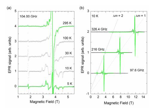
Figure 4. (a) The temperature dependence of the EPR spectra measured at 104.00 GHz and (b) the frequency dependence of the high-frequency EPR spectra at 10 K. The solid green lines are fits of the  $Cr^{III} \cdots Cr^{III}$  dimer model (see text for details).
