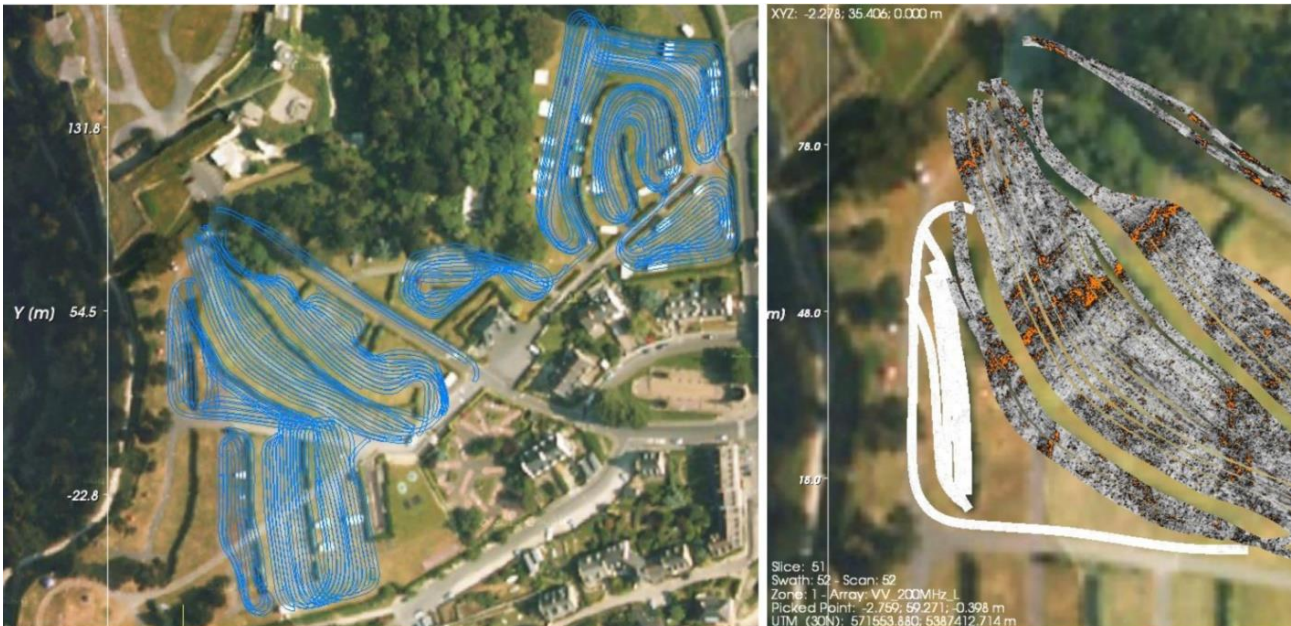
Figure 12: Area in Alet covered with the GPR and results in the southwest zone with z = -0.4 m.
