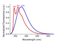
Figure 23. Normalized Absorption (left) and emission (right,  $\lambda_{exc}$ : 309 nm) spectra of **4-PhCbz-SBF** (red lines) and of **4-Ph(OMe)<sub>3</sub>-SBF** (blues lines) recorded in cyclohexane, C:  $10^{-6}$ M
