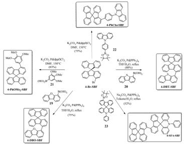
Figure 21. Synthesis of 4-DBF-SBF, 118 4-DBT-SBF, 119 4-PhOMe<sub>3</sub>-SBF, 95 4-PhCbz-SBF and 4-SFA-SBF 120
