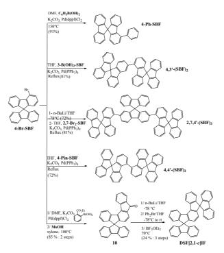
Figure 9. Synthesis of **4-Ph-SBF**, **4,3'-(SBF)**<sub>2</sub>, **2,7,4'-(SBF)**<sub>3</sub>, **4,4'-(SBF)**<sub>2</sub>, **DSF[2,1-c]IF** from **4-Br-SBF**
