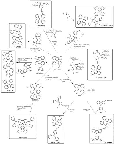
Figure 25: Synthesis of 4-EPHDB-SBF, 94 4-T-DKPP-SBF<sub>2</sub>, 124 4-EPHDBA-SBF, 4-VCbz-SBF, 126 4-VTPA-SBF, 126 DSBF-DPA, 121 DSBF-AP, 123 and 4-AP-SBF<sup>122</sup>
