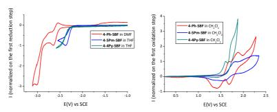
Figure 18. Cyclic voltammetry in reduction (left, recorded in DMF or THF + 0.1 M  $Bu_4NPF_6$ ) and in oxidation (right, recorded in  $CH_2Cl_2 + 0.2$  M  $Bu_4NPF_6$ ) of **4-Ph-SBF** (red line), **4-5Pm-SBF** (blue line) and **4-4Py-SBF** (green line). The current is normalized at the first oxidation or reduction step. (Pt disk electrode  $\emptyset$ 1 mm, 100 mV/s).
