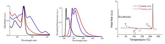
Figure 12. Absorption (left) and Emission (middle) spectra of **4-Ph-SBF** (red line), **DSF[2,1-c]IF** (blue line) and **SBF** (back line) in cyclohexane, C=10<sup>-6</sup> M, DSC curves of **4-Ph-SBF** (right).
