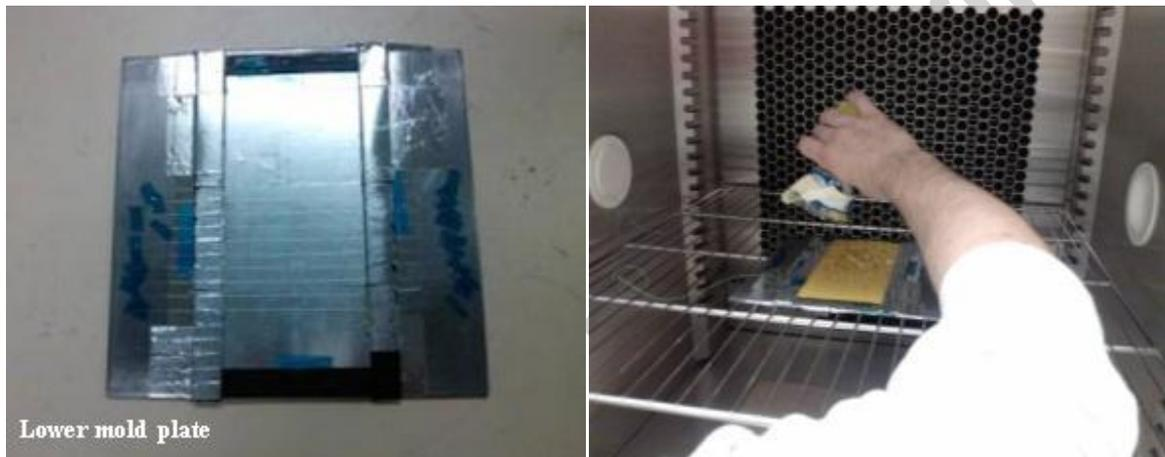
Figure1. Preparation of mold plate (A) and mold position in the heating chamber (B).
