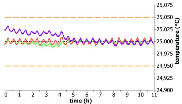
**Figure 2.** Temperature graph for the stabilization at the temperature of 25°C at the points 1 (violet), 2 (red) and 3 (green) near the cavity, see Fig. 1. With small gradient at the beginning, all temperatures stabilize to the required values in several hours. Orange lines show the deviation from the setting point by 50 mK, which corresponds to the accuracy of the measurement.
