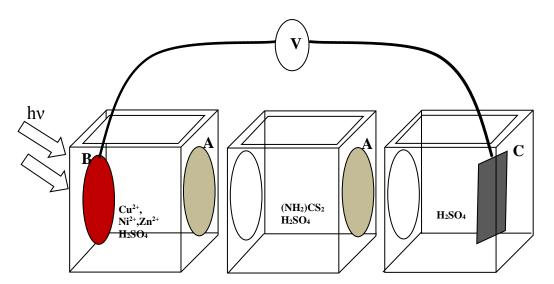
**Figure 2.** Transport cell scheme: **A**: Synthetic membrane; **B**: FeAl<sub>2</sub>O<sub>4</sub> electrode; **C**: platinum electrode
