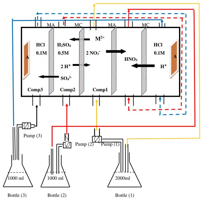
**Figure 1.** The device of closed cell with the capacity of the various compartments AM: anionic membrane; CM: cationic membrane; A: electrode
