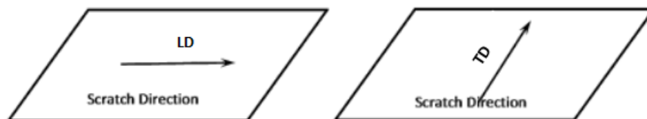
Figure 4. Schematic illustration of longitudinal and transversal orientation of scratch.
