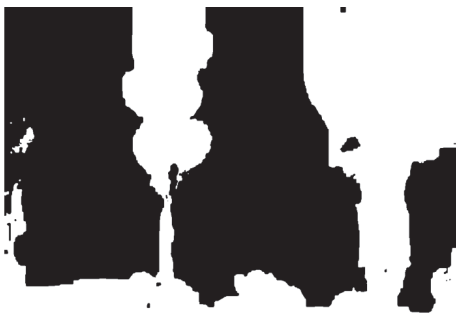
FIGURE 7: Original input binary depth mask of Balloons view 5 frame 1 (1024 × 768 pixels) for foreground zone with Z_{in,l} = 128 , Z_{in,h} = 255 .
