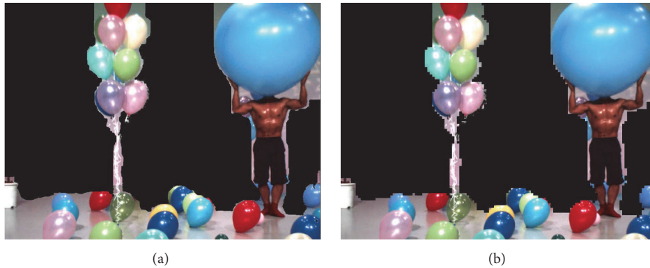
FIGURE 20: Extracted region of interest from texture coded with RoI using (a) the full-resolution DoI-Mask and (b) 8 \times 8 block resolution DoI-Mask.
