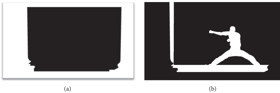
FIGURE 10: Original input binary depth mask of UndoDancer view 1 frame 250 ( 1920 \times 1080 pixels) (a) for foreground zone with Z_{in,l} = 128 , Z_{in,h} = 255 and (b) for depth zone within Z_{in,l} = 100 , Z_{in,h} = 121 .
