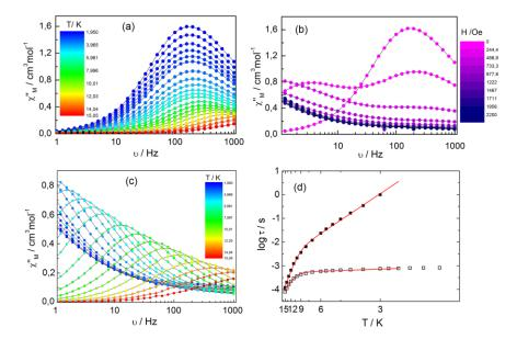
Figure 4. (a) Frequency dependence of χм" between 2 and 15 K, (b) Scan field of the frequency dependence of χм" at 2 K, (c) Frequency dependence of χм" between 2 and 15 K under an applied magnetic field of 1000 Oe;
