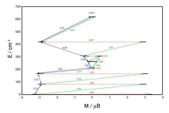
**Figure 7**. Computed magnetization blocking barrier in complex **1** for the Dy<sup>III</sup> ion. Numbers provided on each arrow are the mean absolute values for the corresponding matrix elements of the magnetic transition dipole moment.
