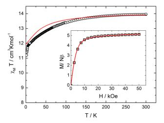
Figure 3. Temperature dependence of  $\chi_MT$  for 1 (black circles). In inset the field variations of the magnetization at 2 K. Full red lines correspond to the simulated curve from ab initio calculations.
