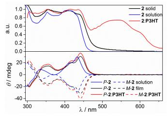
Figure 3. UV-Vis absorption spectra (top) of 2 in solution (blue), as spin-cast films (black) and blended with **P3HT** (red). ECD spectra (bottom) of corresponding enantiomers *P*-(solid line) and *M*-(dashed line) in solution (blue), as spin-cast films (black) and blended with **P3HT** (red).
