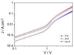
Figure 4. Electron mobility  $\mu_{\rm e}$  of rac-(blue), P-(black) and M- (red) 2 based devices.
