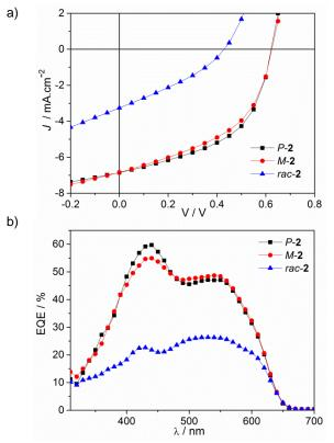
Figure 2. Current density-voltage characteristics (a) and EQE spectra (b) of inverted *rac*-2 (blue), *P*-2 (black) and *M*- (red) 2 based OPV devices.
