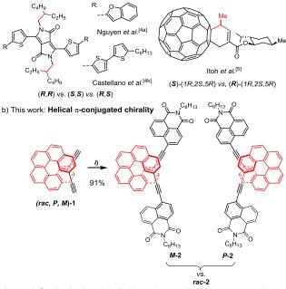
2,15-bisethynyl[6]helicene (1) as either *rac*-1, *P*-1 or *M*-1 was engaged in a Sonogashira cross-coupling reaction, with an excess of 6-bromo-2-hexyl-1*H*-benzoisoquinoline-1,3(2*H*)-dione, affording respectively *rac*-, *P*- and *M*-naphthalimide end-capped helicene derivatives (*rac*-2, *P*-2 and *M*-2) as bright yellow solids in excellent yields (see Supporting Information, SI). This simple
