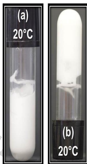
Figure 10: Photographs of foams taken 30 minutes after foam generation at 20^\circ\text{C} below the solubility boundary of the system. Foam did not flow when the vial is inverted. Reprinted with permission from [35]. Copyright 2015 American Chemical Society.
