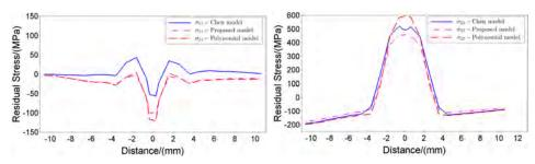
(a) Residual stresses of transversal direc- (b) Residual stresses of longitudinal dition rection
