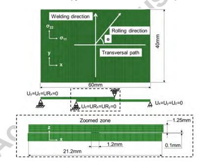
Figure 1: Mesh and geometry of numerical model
