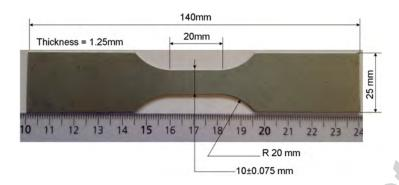
Figure 10: Dimensions of specimen for tensile test
