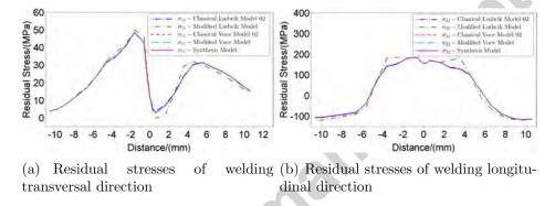
Figure 5: Residual stresses of different hardening models along transversal path
