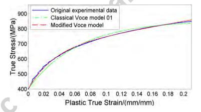
Figure 3: Comparison of Voce model and experimental DP600 data
