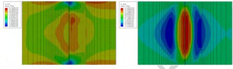
(a) Contour of residual stress  $\sigma_{11}$  of (b) Contour of residual stress  $\sigma_{22}$  of lontransversal direction gitudinal direction
