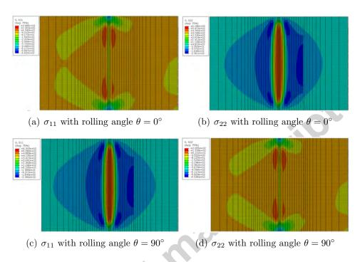
Figure 12: Contour of residual stresses with different material rolling orientations
