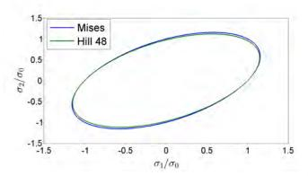
Figure 11: Yield surface predicted by Hill48 anisotropic model and Von Mises criterion
