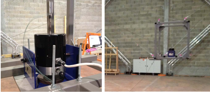
Fig. 5. Electro-dynamic shaker mounted on the end-effector of CoGiRo.
