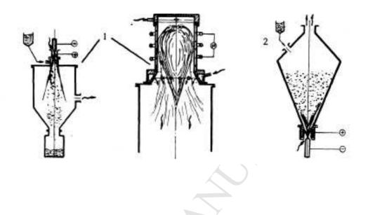
Fig. 19 Schematic diagram of plasma centrifugal furnace for metallurgical application.
