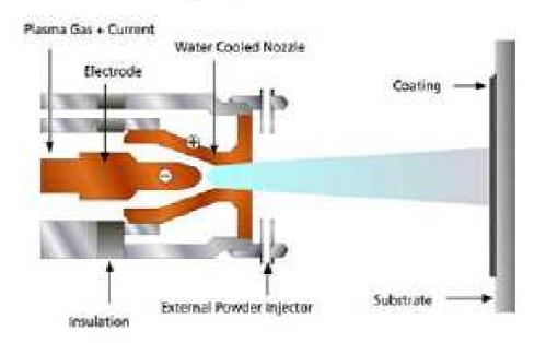
Fig 15 A schematic diagram of thermal plasma coating.
