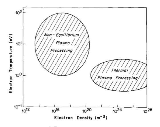
Fig. 2. Typical ranges of electron temperature range with elctron density for non equilibrium and equilibrium plasma processing system.
