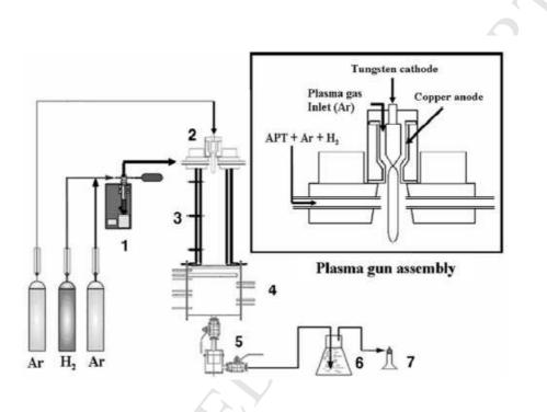
Fig. 18 Schematic diagram of plasma gun assembly for nano particle fabrication.
