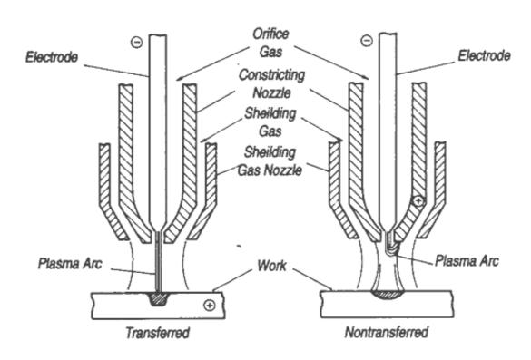
Fig. 7 Schematic diagram of transferred and non transferred arc reactors.
