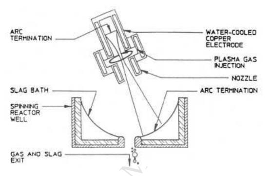
Fig. 16. Plasma technique for slag metallurgy.
