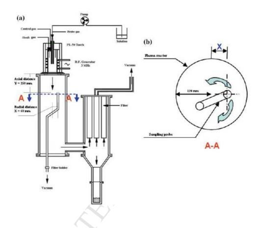
Figure 17 (a) RF plasma installation for RF-ICTP synthesis process.
