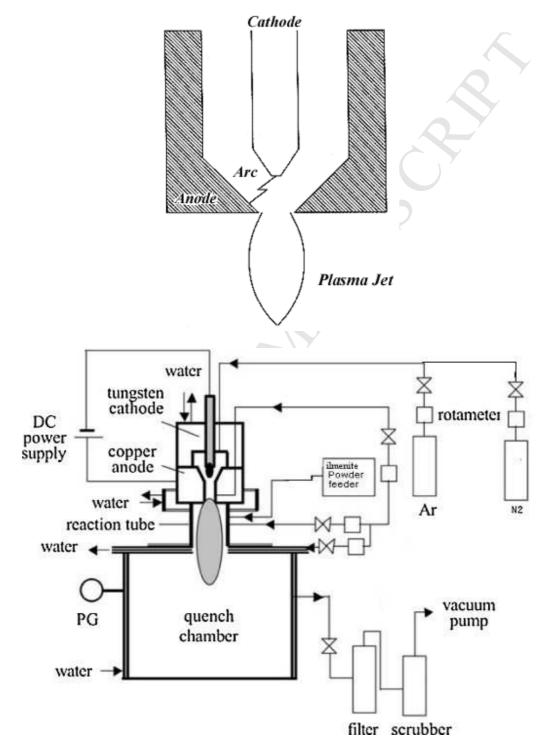
Fig. 8 Schematic diagram and example of non transferred arc reactor.
