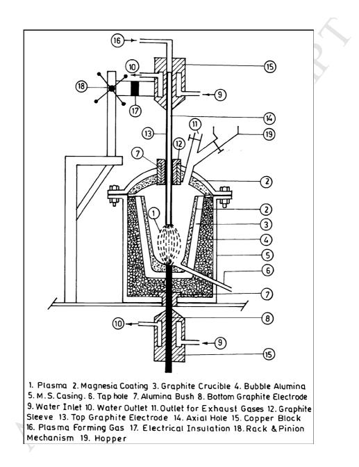
Fig. 10 Schematic diagram of transferred arc reactor of thermal plasma process: inflight direct current extended arc plasma reactor.
