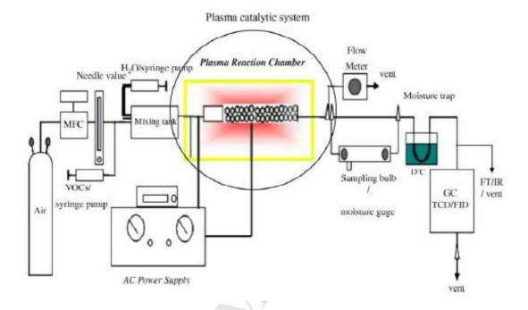
Figure 13 Schematic representation of discharge plasma reactor apparatus.
