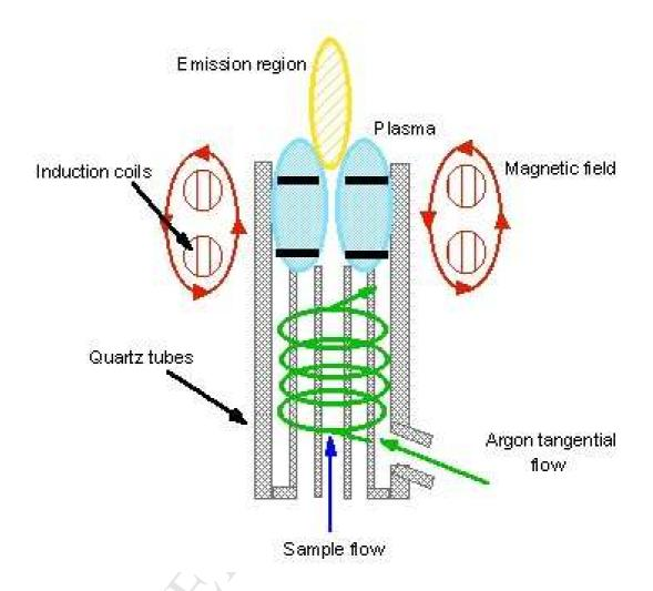
Fig. 12 Schematic diagram of RF inductively coupled discharge
