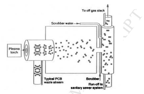
Fig. 14 Schematic diagram of pyrolysis unit for waste treatment.
