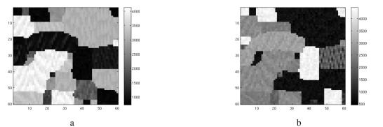
Figure 1. Illustration of component images p = 45 ( $\lambda = 639.75$  nm) (a) and p = 100 ( $\lambda = 898.68$  nm) (b)
