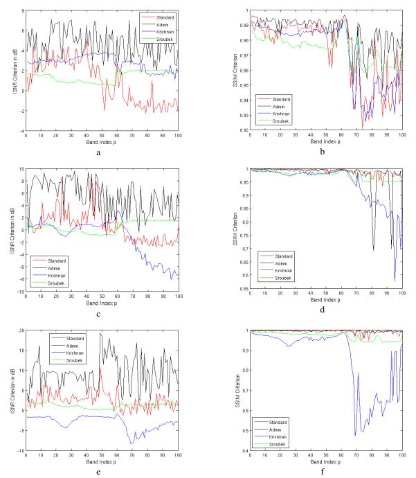
Figure 4. ISNR (left column) and SSIM (right column) values obtained in each spectral band for each of the four methods. First row (a) and (b) is for defocusing blur (d = 7), second row (c) and (d) for Gaussian Blur ( $\sigma = 2$ ) and third row (e) and (f) for Linear Motion Blur ( $l = 7, \theta = 135^{\circ}$ ).
