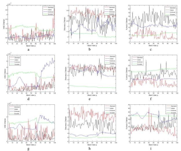
Figure 5. Mean Squared Error (left column), skewness (middle column) and kurtosis (right column) properties of the PSF estimation error bias experimental distribution in each spectral channel for each of the four methods. First row (a) - (c) is for defocusing blur (d = 7), second row (d) - (f) for Gaussian blur ( $\sigma = 2$ ) and third row (g) - (i) for linear motion blur ( $l = 7, \theta = 135^{\circ}$ ).
