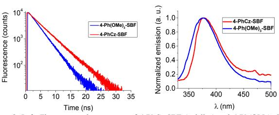
**Figure 8.** Left: Fluorescence decay curves of **4-PhCz-SBF** (red line) and **4-Ph(OMe)<sub>3</sub>-SBF** (blue line) in cyclohexane ( $\lambda_{exc}$ = 300 nm,  $\lambda_{em}$ = 375 nm), right: solid state emission of **4-PhCz-SBF** (red line,  $\lambda_{exc}$ = 280 nm) and **4-Ph(OMe)<sub>3</sub>-SBF** (blue line,  $\lambda_{exc}$ = 280 nm).
