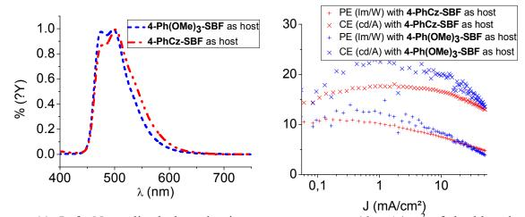
**Figure 11.** Left: Normalized electroluminescent spectrum at 10 mA/cm<sup>2</sup> of the blue devices using **4-PhCz-SBF** (red) or **4-Ph(OMe)<sub>3</sub>-SBF** (blue) as host doped with FIrpic (17-20% in mass) as emitting layer; right: Current efficiency (CE, Cd/A, ×) and power efficiency (PE, lm/W, +) versus current density of the green devices using **4-PhCz-SBF** (red) or **4-Ph(OMe)<sub>3</sub>-SBF** (blue) as host doped with FIrpic (17-20% in mass) as emitting layer
