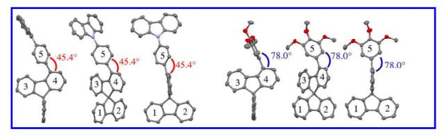
**Figure 2.** Different views of molecular structures of **4-PhCz-SBF** (left) and of **4-Ph(OMe)<sub>3</sub>-SBF** (right) obtained by X-Ray diffraction on single crystals
