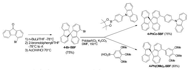
Scheme 1. Synthesis of 4-Ph(OMe)<sub>3</sub>-SBF and of 4-PhCz-SBF.
