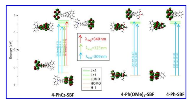
**Figure 5**. Representation of the energy levels and the main molecular orbitals involved in the electronic transitions of **4-PhCz-SBF** (left), **4-Ph(OMe)<sub>3</sub>-SBF** (middle) and **4-Ph-SBF** (right) obtained by TD-DFT M06-2X/6-311+G(d,p), shown with an isovalue of 0.04 [e bohr<sup>-3</sup>]<sup>1/2</sup>. For clarity purpose, only the main contribution of each transition is shown (see SI for details).
