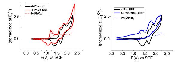
**Figure 3.** Cyclic voltammetry at 100 mVs<sup>-1</sup> in CH<sub>2</sub>Cl<sub>2</sub>/[NBu<sub>4</sub>][PF<sub>6</sub>] 0.2 M in the presence of **4-Ph-SBF** (black line), **4-PhCz-SBF** (red line), **N-PhCz** (red dotted line), **4-Ph(OMe)<sub>3</sub>-SBF** (blue line) and **Ph(OMe)<sub>3</sub>** (blue dotted line).
