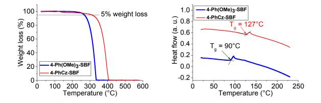
Figure 1. TGA (left) and DSC curves (right) of 4-Ph(OMe)<sub>3</sub>-SBF (blue line) and of 4-PhCz-SBF (red line).
