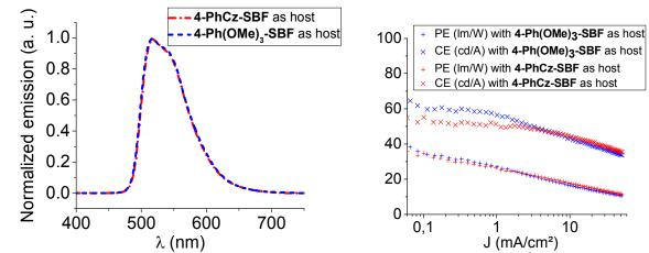
**Figure 10.** Left: Normalized electroluminescent spectrum at 10 mA/cm<sup>2</sup> of the green devices using **4-PhCz-SBF** (red) or **4-Ph(OMe)<sub>3</sub>-SBF** (blue) as host doped with  $Ir(ppy)_3$  (10% in mass) as emitting layer; right: Current efficiency (CE, Cd/A, ×) and power efficiency (PE, Im/W, +) versus current density of the green devices using **4-PhCz-SBF** (red) or **4-Ph(OMe)<sub>3</sub>-SBF** (blue) as host doped with  $Ir(ppy)_3$  (10% in mass) as emitting layer.
