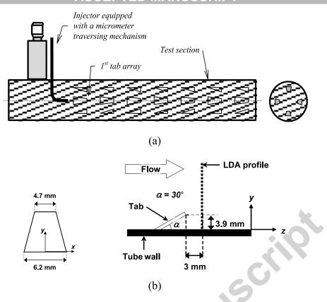
**Fig. 3.** (a) Longitudinal view of the test section with seven aligned rows of baffles. The injector is a 3-mm tube placed in the centre of the continuous phase flow. (b) Dimensions of mixing tab: front view, side view and position of LDA radial profile.
