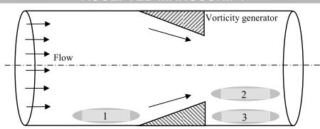
Fig. 6. Distribution of turbulent kinetic energy in the flow with vorticity generator: high ACCEPTED TO THE PROPERTY OF TH velocity core region (1), high shear zone (2) and tab wake (3).
