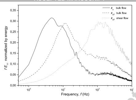
Fig. 7. Normalized premultiplied spectra downstream from the seventh row of baffles (location  $X_{o7}$ ) for two radial locations (shear region and bulk flow) compared with upstream spectrum (location  $X_{o}$ ) for the bulk flow. Re = 15000.
