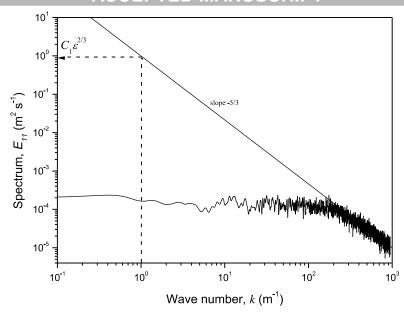
Fig. 8. Determination of the  $C_1 \, \varepsilon^{2/3}$  value, for Re=15000, downstream from the seventh row of baffle in bulk flow.
