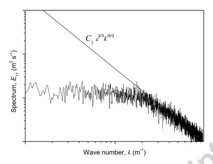
**Fig. 2.** Turbulent spectra and extrapolation of the inertial zone. Numerical values are deliberately erased to exhibit the general behaviour of the plot.
