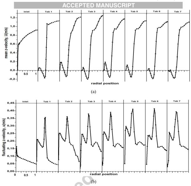
**Fig. 5.** Experimental velocity profiles along a radial line 3 mm behind each vorticity generator: (a) mean axial velocity, (b) fluctuating z-velocity component of axial velocity.
