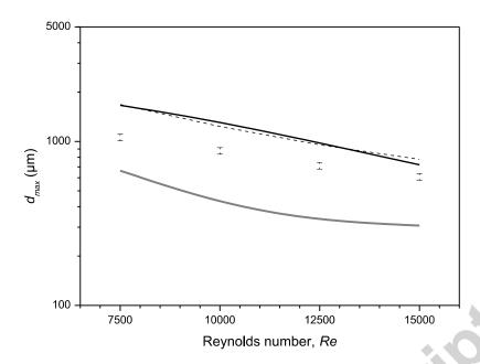
**Fig. 11.** Experimental  $d_{max}$  with oil volume fractions 2.5 % to 15 % ( $\square$ ). Theoretical  $d_{max}$  computed by TS model from Eq. (12) with  $C_1 \varepsilon^{2/3}$  value obtained from spectra in the outlet section: ( $\longrightarrow$ ) in bulk zone, ( $\longrightarrow$ ) in shear zone. Theoretical  $d_{max}$  computed by HK model from Eq. (11) with the mean dissipation rate in the device ( $\longrightarrow$ ).
