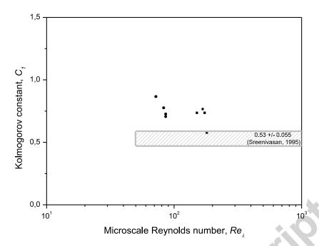
**Fig. 9.** Experimental Kolmogorov constant  $C_1$  ( $\circ$ ) upstream in the bulk zone, ( $\bullet$ ) downstream in the bulk zone, ( $\blacksquare$ ) downstream in the shear zone.
