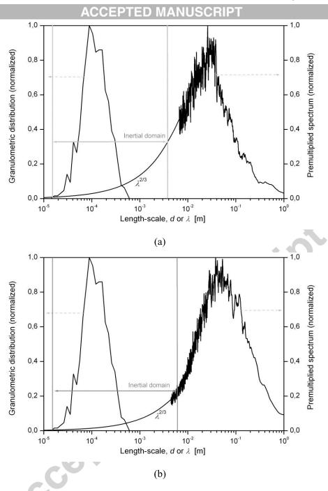
**Fig. 10.** Comparison between drop size distribution and turbulent spectra: (a) spectrum in the bulk zone, (b) spectrum in the high shear zone. The normalized premultiplied spectra are taken at the mixer outlet versus eddy size  $\lambda = U_{conv}/f$ . The premultiplied spectrum is extrapolated by a  $\lambda^{2/3}$  trend curve. The inertial domain is positioned on the graph. Re = 15000 and oil fraction 5 %.
