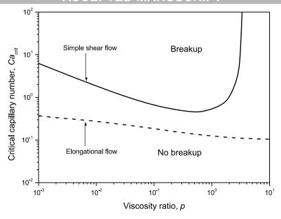
Fig. 1. Critical capillary number (adapted from Grace, 1982).
